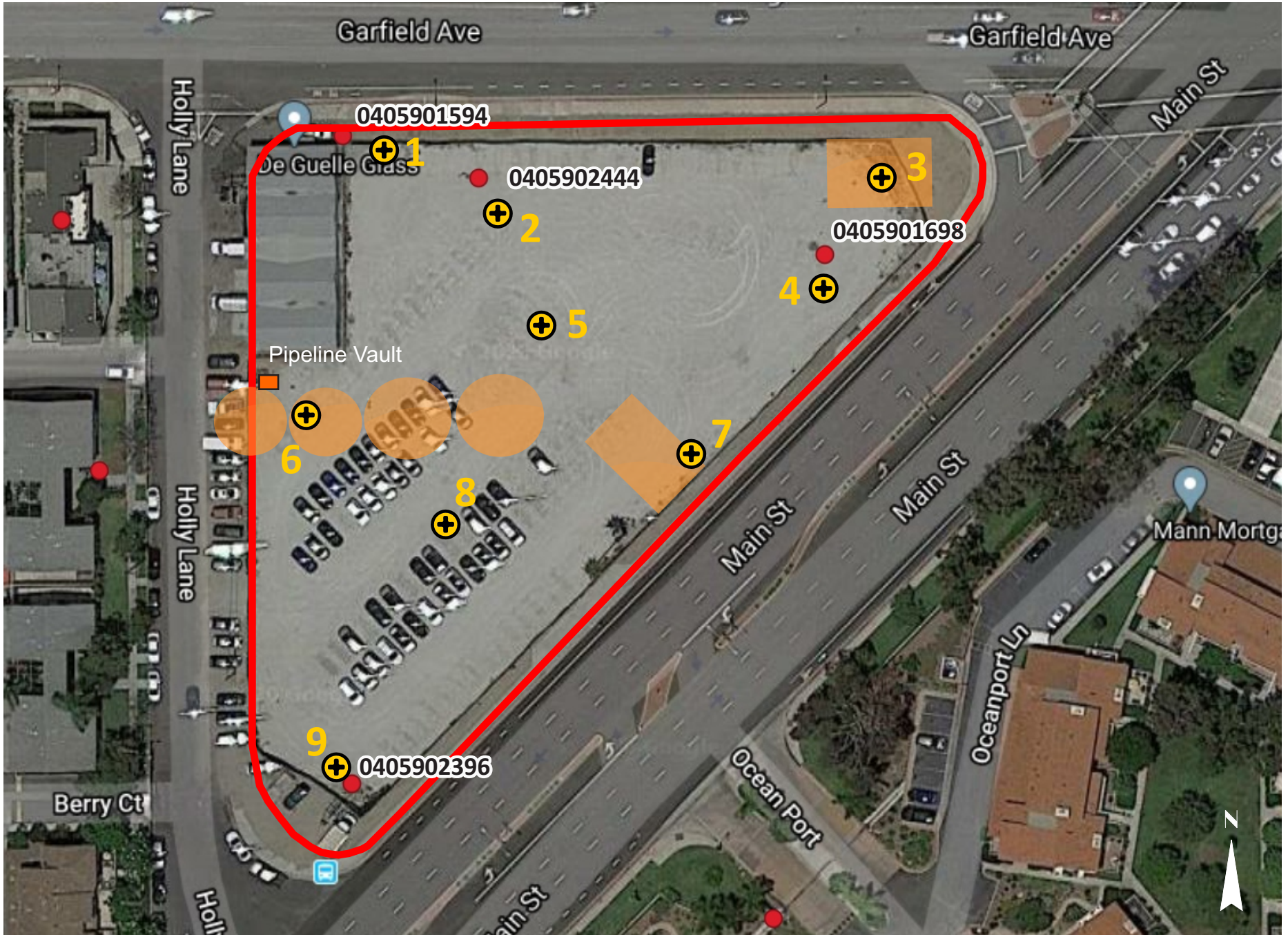
Figure 5 - Investigation Probe Locations
