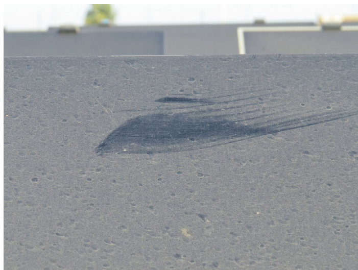
Photo 6: Wing marks on PV panel (same pictured above) from impact by American coot
