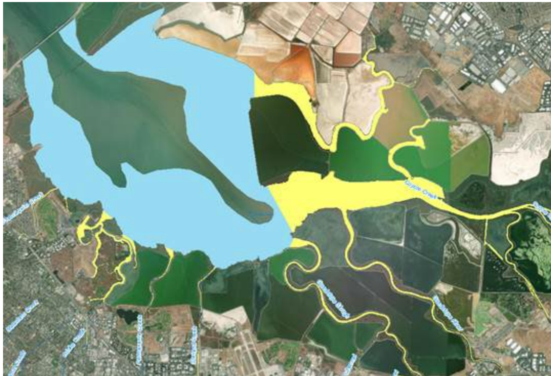
FIGURE 1: Approximate South Bay Estuary Boundary at Mean Sea Level. Tidal Flat (blue) and Riverine Tidal Prism (Yellow)
