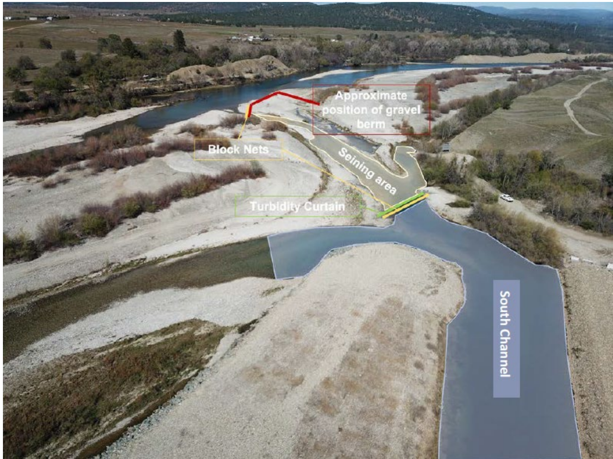
Figure 6. Example of where fish avoidance measures were used in 2022 prior to excavations.
