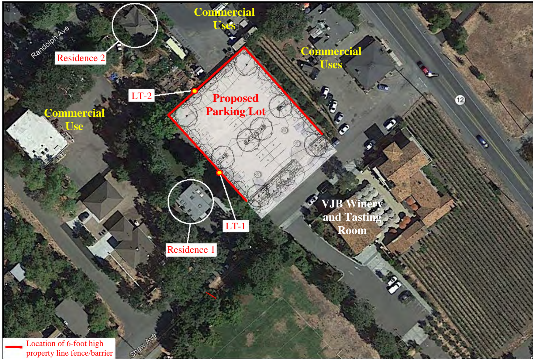
Figure 1: Site Plan Showing Noise Monitoring Locations, Nearby Land Uses, and Receptor Locations
