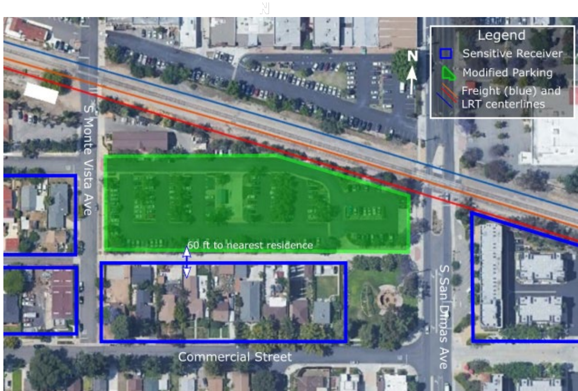
Figure 21: Aerial Map of Proposed Modified Parking Lot and the Nearest Noise-Sensitive Receiver for San Dimas Station
