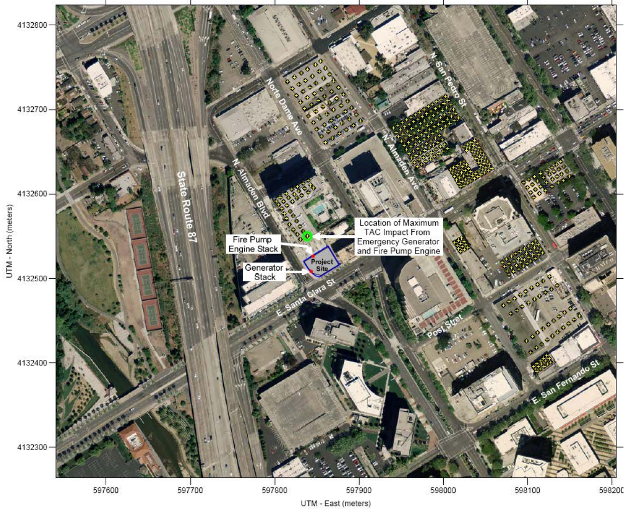
Figure 2. Project Site, Locations of Emergency Generator and Fire Pump Stacks, Off-Site Sensitive Receptors and Location of Maximum TAC Impacts
