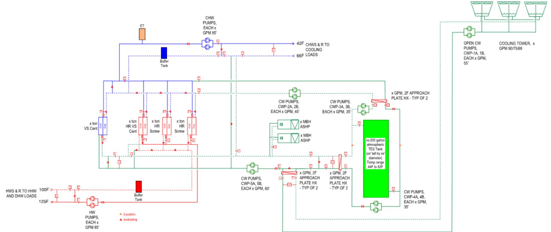
Figure 7 – Central Plant Schematic from Taylor Engineering
