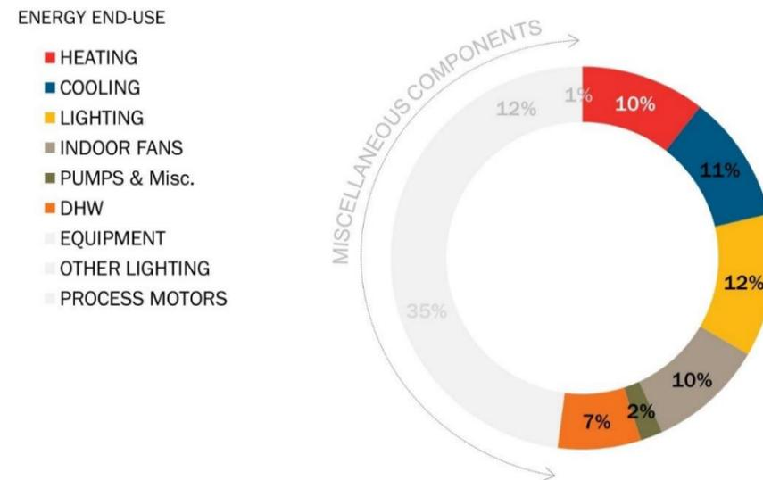
Figure 4a - Proposed Design Energy Use TDV Characterization
