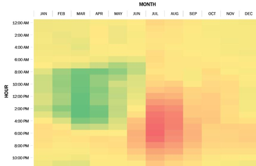
Figure 13 - Annual Marginal Greenhouse Gas Emissions Profile for CAISO, Relative CO2lbs/kWh electricity
