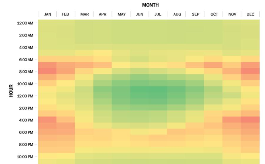
Figure 16 - Annual Marginal Greenhouse Gas Emissions Profile for Fountain Alley, with Maximum PV array. Relative CO2lbs/kWh electricity
