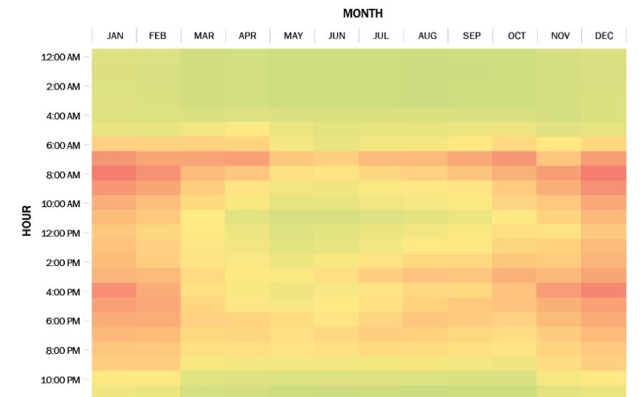
Figure 15 - Annual Marginal Greenhouse Gas Emissions Profile for Fountain Alley, with Moderate PV array. Relative CO2lbs/kWh electricity
