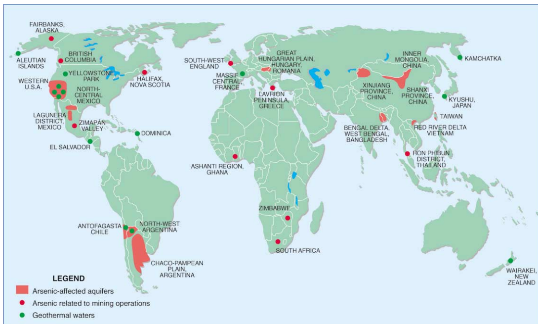
Fig. 3. Distribution of documented world problems with As in groundwater in major aquifers as well as water and environmental problems related to mining and geothermal sources. Areas in blue are lakes.
