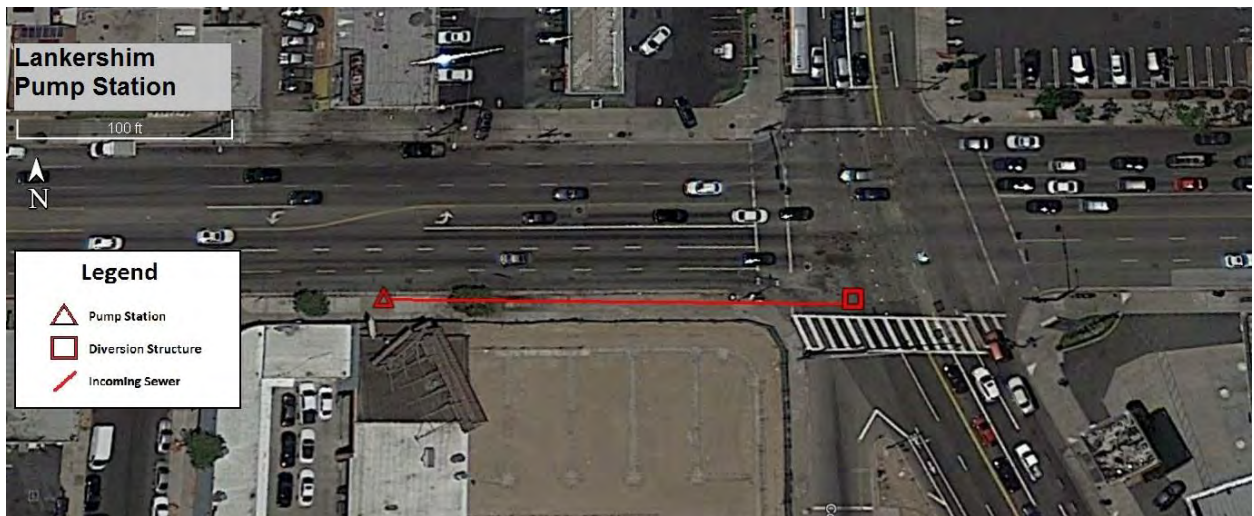
Figure 5. Pump stations and diversion structures located along Victory Boulevard
