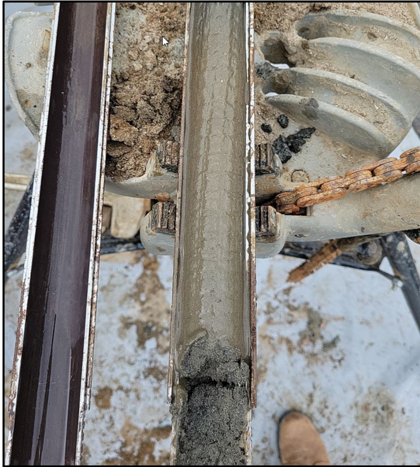
Figure 4-3. Bay Sediments in Boring B-1
