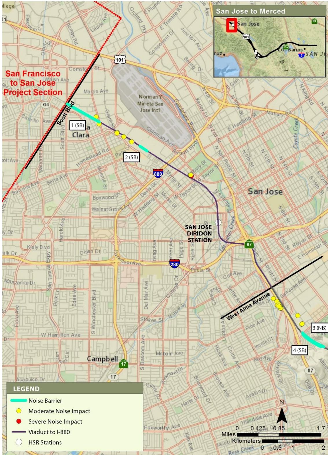
Figure 3.4-33 Proposed Noise Barriers and Residual Noise Impacts—Alternative 1 (San Jose Diridon Station Approach Subsection)
