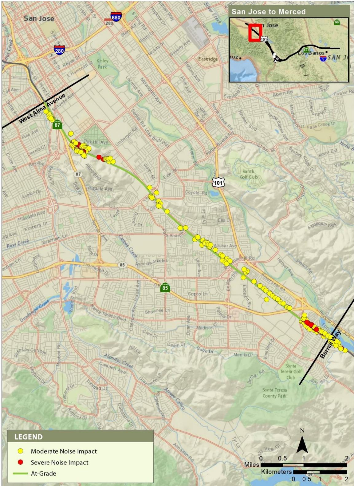
Figure 3.4-14 2040 Plus Project Noise Impacts—Alternative 2 (Monterey Corridor Subsection)
