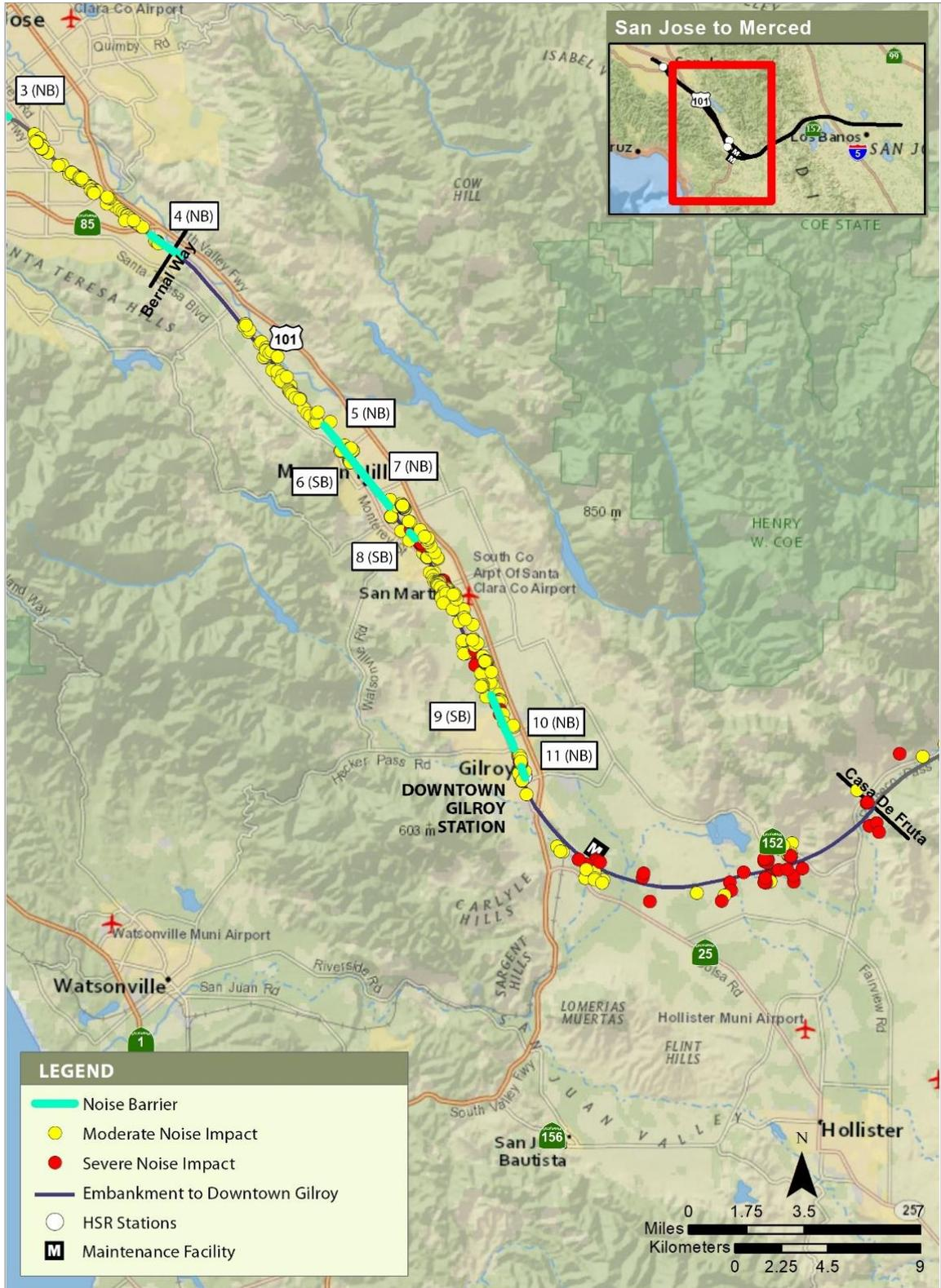
**Figure 3.4-37b Proposed Noise Barriers and Residual Noise Impacts—Alternative 2 with the Tunnel Design Variant (Morgan Hill and Gilroy Subsection)**
