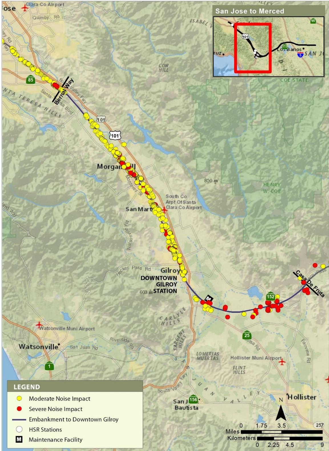
**Figure 3.4-15b 2040 Plus Project Noise Impacts—Alternative 2 with the Tunnel Design Variant (Morgan Hill and Gilroy Subsection)**
