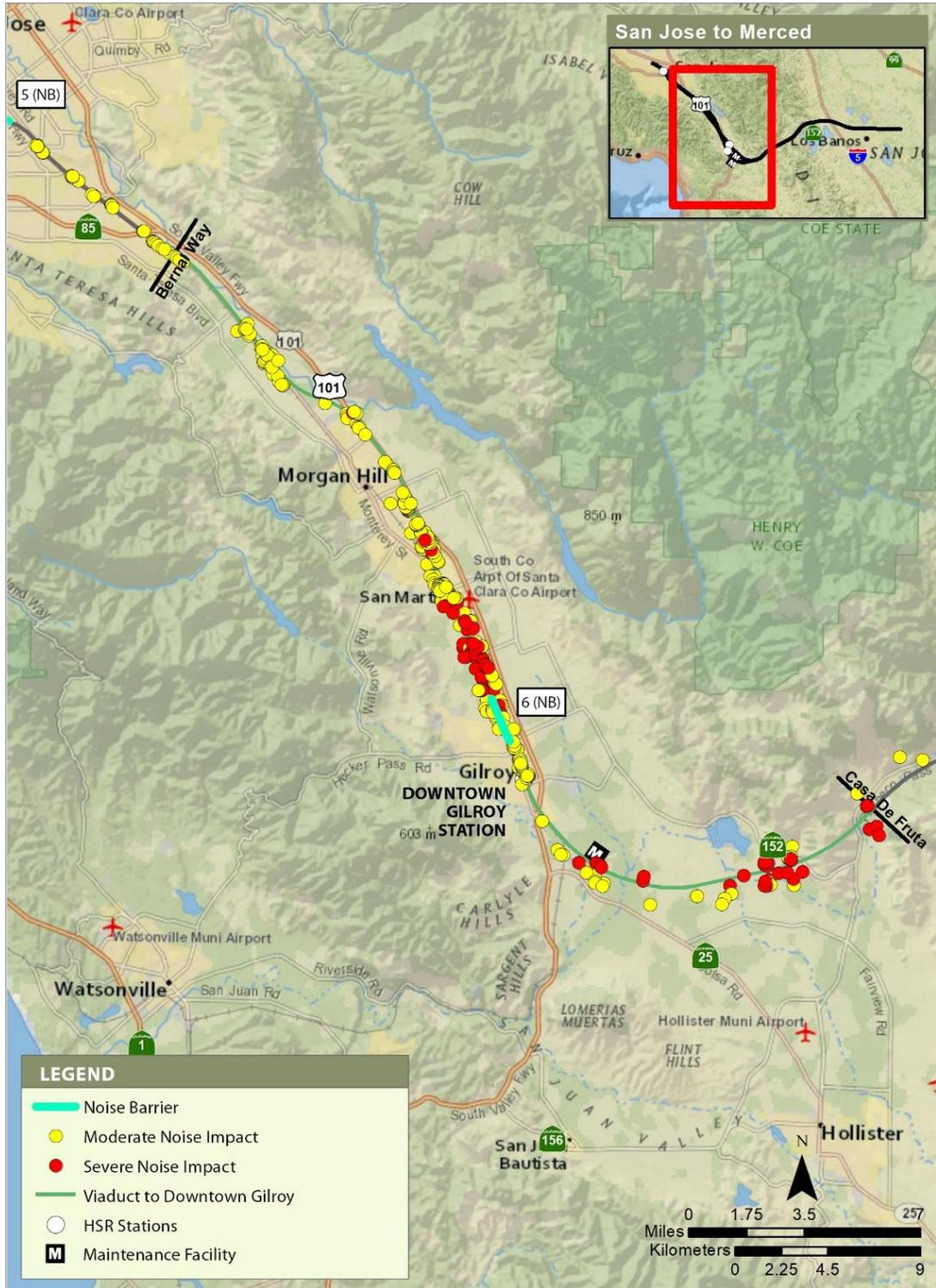
**Figure 3.4-35a Proposed Noise Barriers and Residual Noise Impacts—Alternative 1 without the Tunnel Design Variant (Morgan Hill and Gilroy Subsection)**
