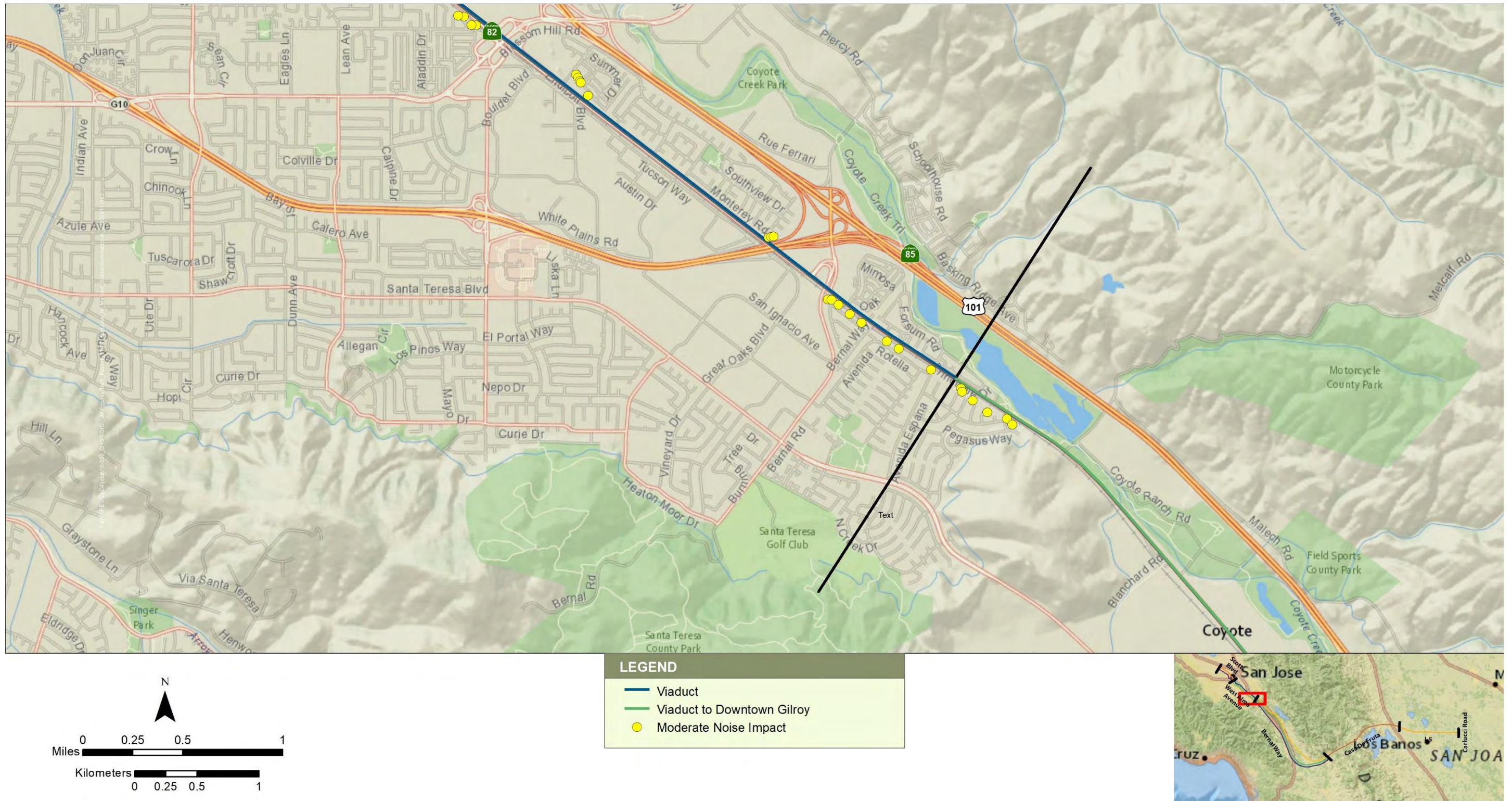
Figure C-5 2040 Plus Project Noise Impacts—Alternative 1
