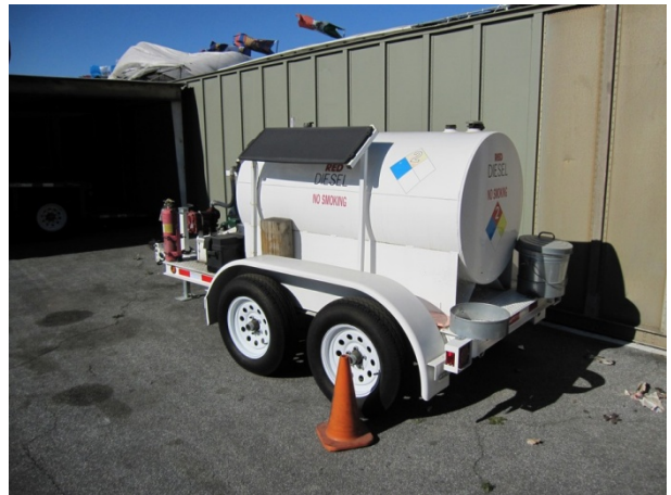
Photograph 8. Trailer mounted diesel AST.
