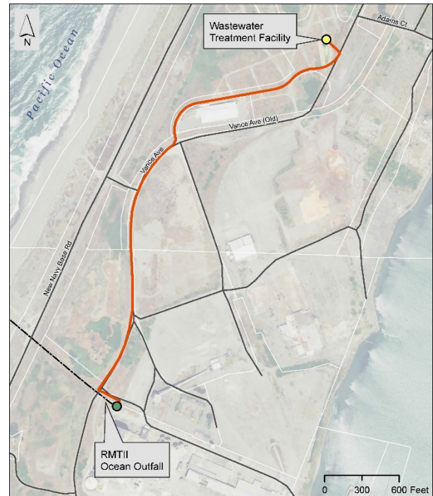
Figure 2-3 Wastewater Disposal Alternative
