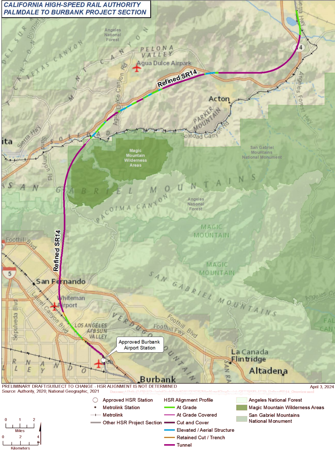
Figure 2-48 Refined SR14 Build Alternative Overview Map
