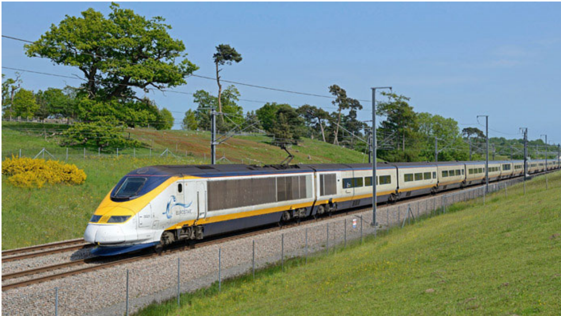
Figure 2-5 Example of At-Grade Profile Showing Contact Wire System and Vertical Arms of Pantograph Power Pickups
