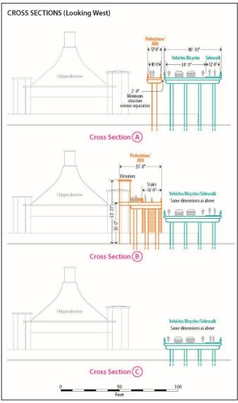
Alternative 8: Wide Pier Bridge Replacement with Vehicle and Bike Lanes and Northside Pedestrian/ADA Path
