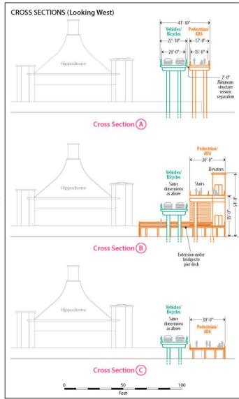
Alternative 7: Wide Pier Bridge Replacement with Vehicle and Bike Lanes and Southside Pedestrian/ADA Path
