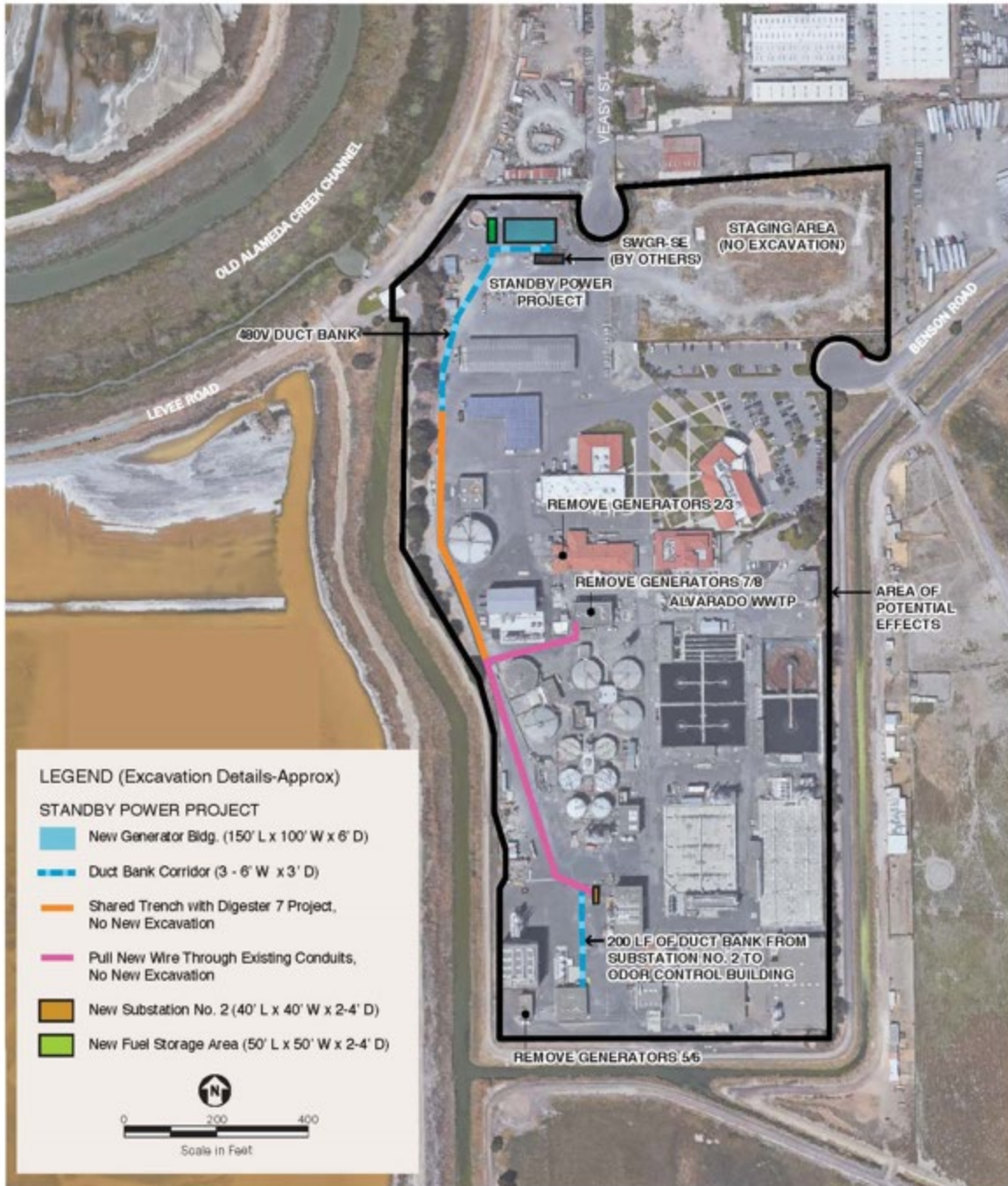
Figure 2. Construction Characteristics of Modified Standby Power Generation System Upgrade Project as Included in this Revised Addendum
