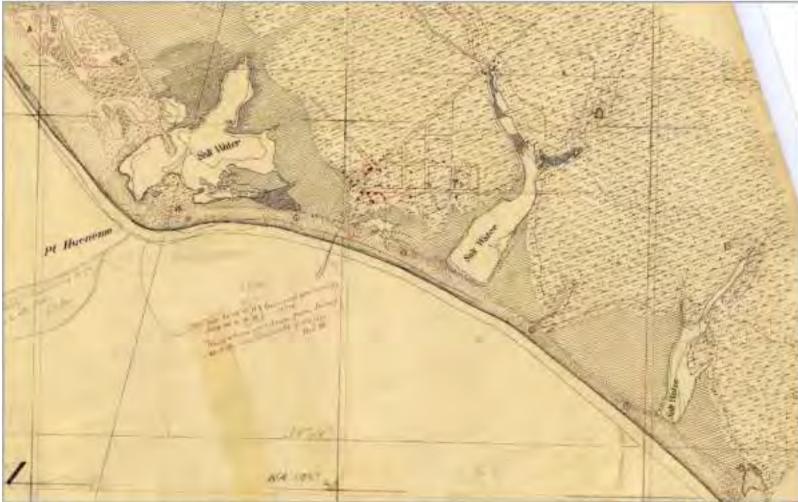
Figure 3. Lagoons south of Point Hueneme as shown on T-sheet 893 (ca. 1857). These lagoons appear to have: 1) formed via downcutting by distributary channels of the Santa Clara River, 2) had the potential to "perch" behind the raised berm and 3) to have had the potential to connect laterally to one another behind the beach berm. Thus when inflow raised water level in one system they may have flowed to adjacent systems.
