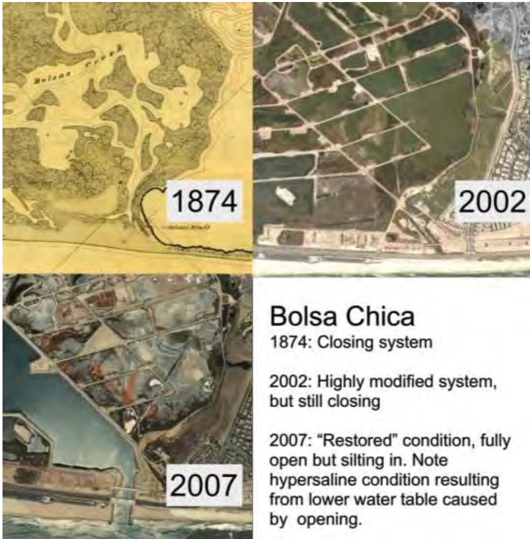
Figure 18. Creation of ahistoric conditions at Bolsa Chica through jettying a perennial deepwater channel. This "restoration" will require frequent and expensive dredging because existing physical processes do not support the fully open condition that was constructed. The areas surrounding constructed wetland appear to be drier and saltier because the water table will have dropped following complete opening.
