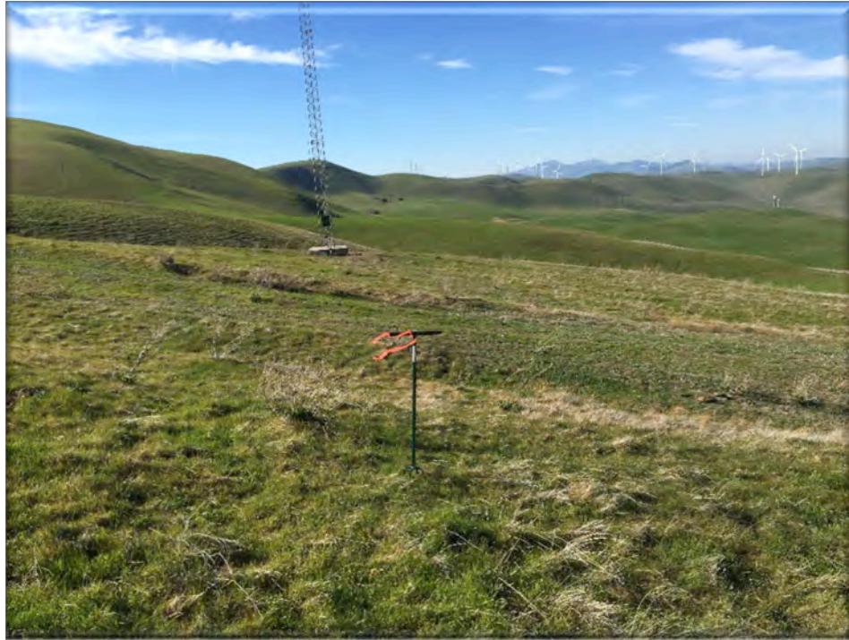
Plate 55. Looking northwest from the initially proposed Turbine 18 location. Note the location on a descending slope; however, the ridge top is generally flat and broad. A meteorological tower is in the background. Also note the higher elevation hills to the west. As birds fly eastward over these hills, they will fly at the altitude of the rotor plane.
