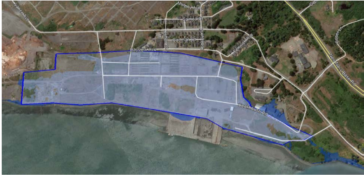
Figure 3. Low-lying waterfront sediment use site (WF-1) that is vulnerable to 1.0 meter of sea level rise (blue shading).
