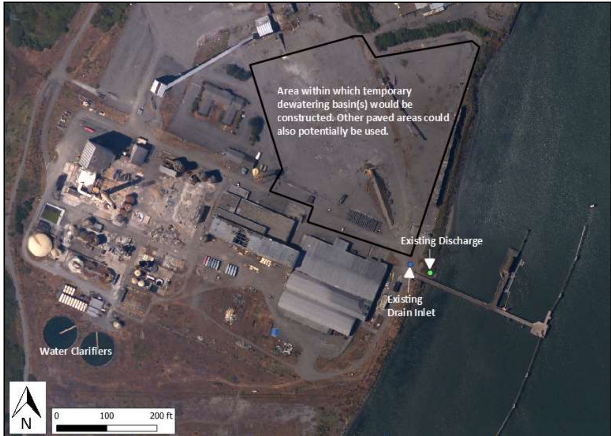
Figure 2.2-6. Potential Temporary Dewatering Basin Site – Redwood Marine Terminal II
