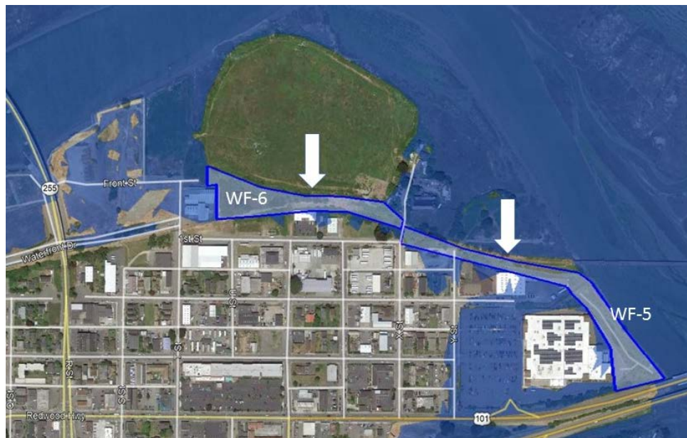
Figure 6. White arrows point to low-lying waterfront sediment use sites WF-5 and WF-6 (polygons with blue boundary and white shading) that could create barriers to tidal inundation of the City of Eureka, which is vulnerable to 1.0 meter of sea level rise (blue shading).
