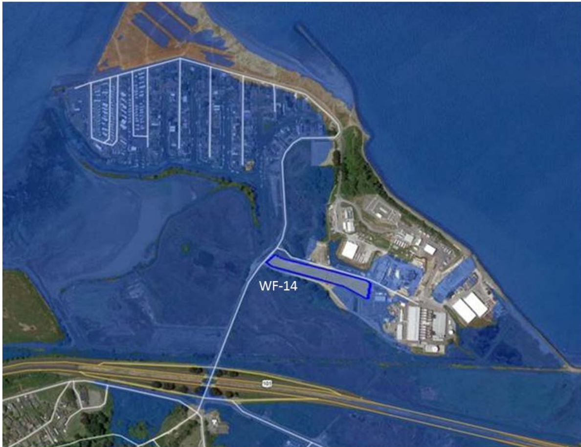
Figure 8. Waterfront sediment use site WF-14 (polygon with blue boundary and white shading) that could block a pathway for tidal inundation of PG&E's property and facilities vulnerable to 1.0 meter of sea level rise MMMW (blue shading).
