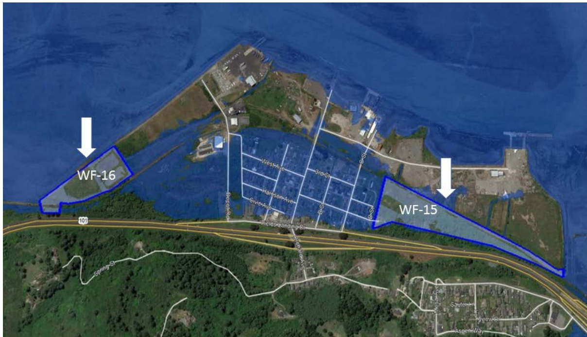
Figure 4. White arrows point to low-lying waterfront sediment use sites WF-15 and WF-16 (polygons with blue boundary and white shading) that could block pathways for tidal inundation of the community of Fields Landing that is vulnerable to 0.5 meters of sea level rise (blue shading).
