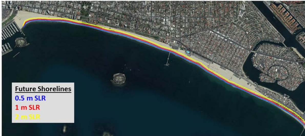
Figure 6: Projected Shoreline Change due to Multiple Sea Level Rise Scenarios Assuming no Future Beach Nourishments
