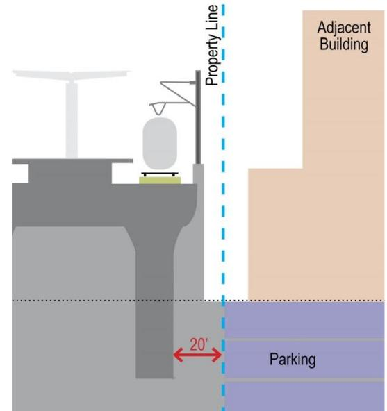
*An underground structure proposed within twenty (20) feet of a Metro structure may require a threat assessment and blast/explosion study.*
