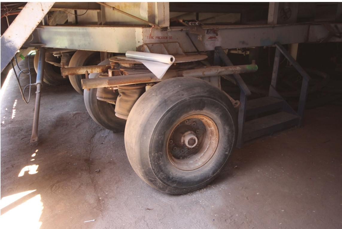
Figure 3-38: The wheels that enable the seating sections to be moved.
