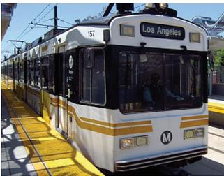
**Metro Rail:** Metro operates heavy rail (HRT) and light rail (LRT) transit lines in underground tunnels, along streets, off-street in dedicated ROW, and above street level on elevated structures. Heavy rail trains are powered by a “third rail” along the tracks. Light rail vehicles are powered by overhead catenary systems (OCS). To support rail operations, Metro owns and maintains traction power substations (TPSS), maintenance yards, and other infrastructure.
