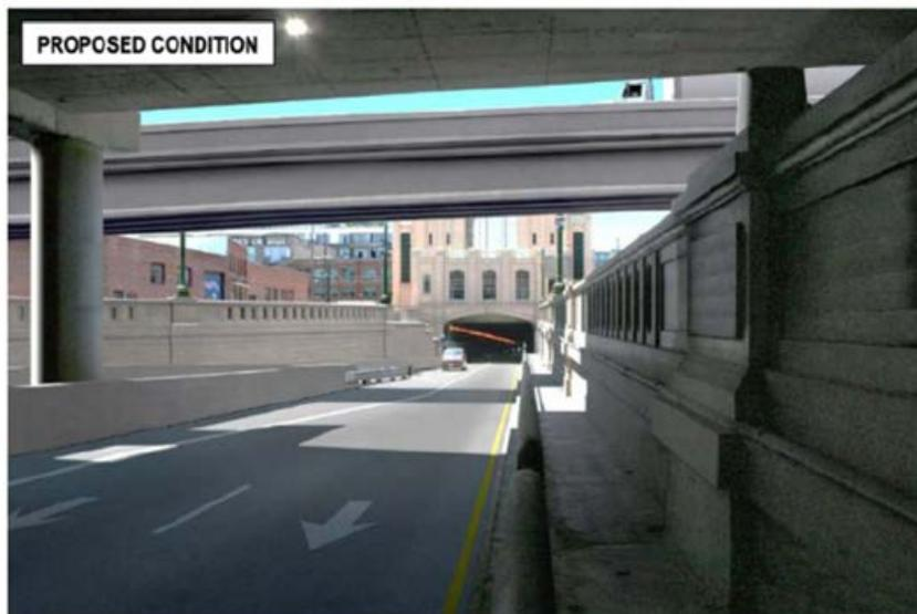
**[Comment O-4-7** To adjust the design, study cutting into the wall to provide the horseshoe without curving it. This would maintain more of the existing wall and the character defining symmetry while allowing the horseshoe to occur.] **[Comment O-4-8** Decrease the size of the shoulder near the historic walls to reduce the amount that would need to be destroyed.] **[Comment O-4-9** The left turn pocket should also be adjusted to save 100 feet of wall near 6th Street.]
