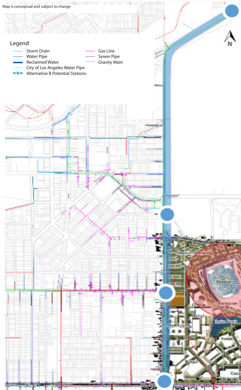
Figure 4.4-6: Utilities along Alternative B: Fairview Heights Alignment
