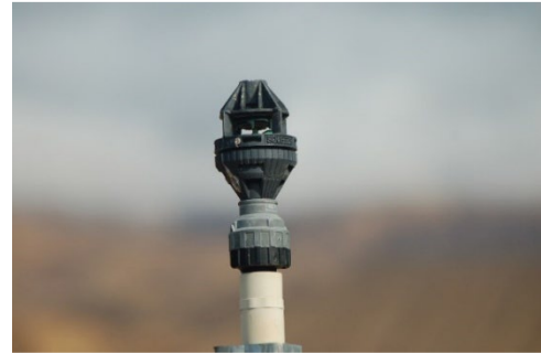
Frost Pond System Sprinkler Emitter
