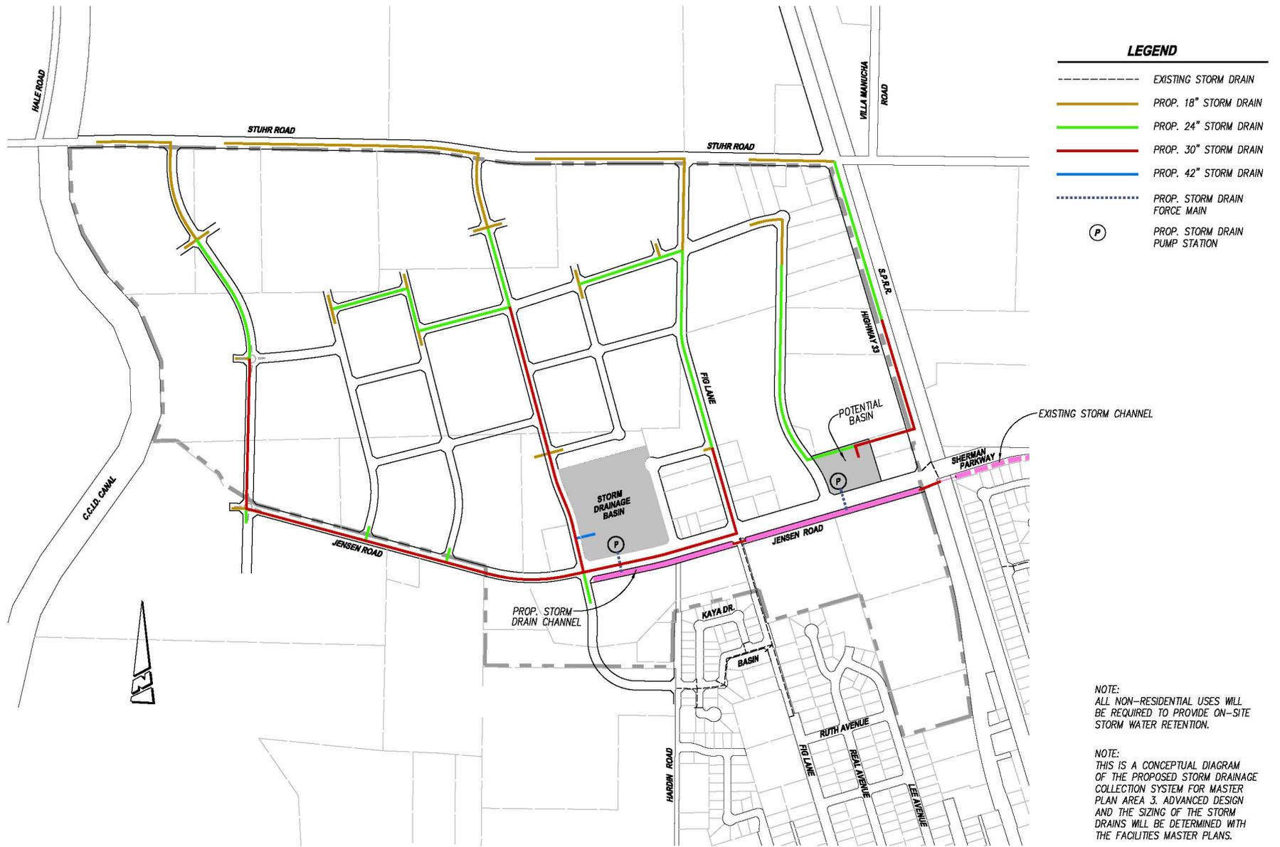
Figure 3.7: Preliminary Backbone Stormwater System Plan
