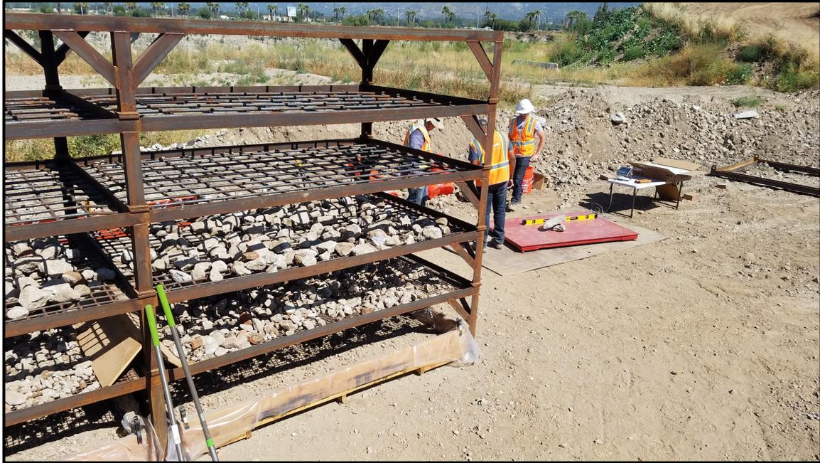
**2017 May** – South-Central Area (Area 2S). Large-scale gradation testing of the blended rubble fill excavated during a bulk density test. View to northwest.
