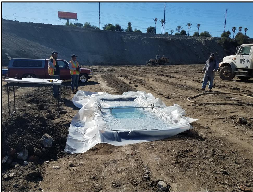
**2017 November** – Southeast Pit (Area 3S). Large-scale bulk density testing of blended rubble fill. Water volume measurement of excavated pit. View to south.
