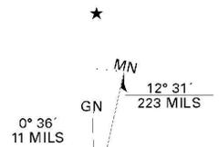
UTM GRID AND 2012 MAGNETIC NORTH DECLINATION AT CENTER OF SHEET
