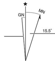
UTM GRID AND 1953 MAGNETIC NORTH DECLINATION AT CENTER OF SHEET
