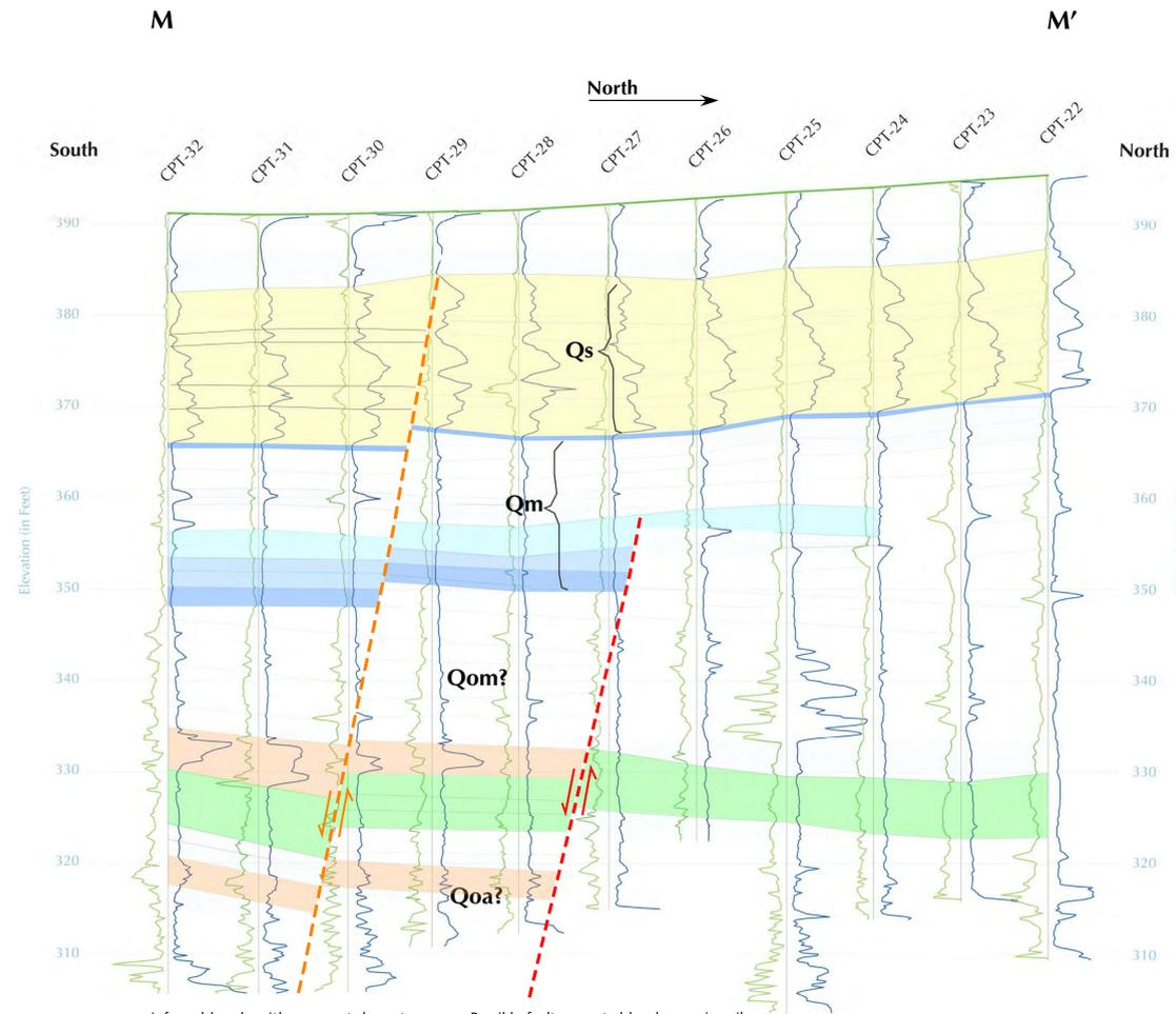
Inferred break, with apparent down-to-the-south vertical displacement required by inclusion of CPT-29. Panel B shows this feature goes away if CPT-29 is not included. Possible fault suggested by changes in soil type at the depth of the Qm and Qom? units. An equally plausible interpretation that does not require a fault in this area is presented in Panel B.
