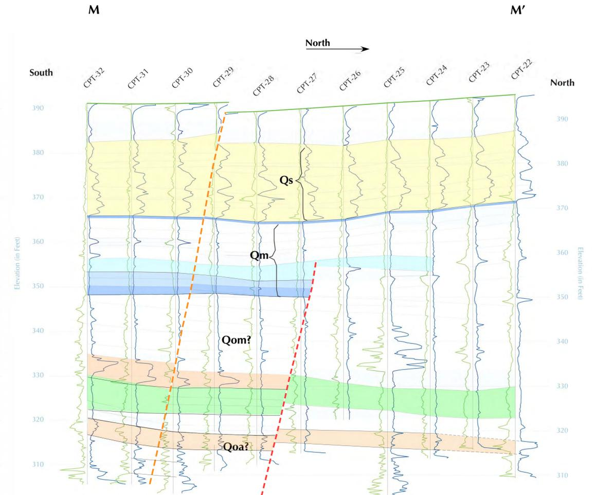
Designation of the geologic units is based on a comparison of the CPT curves from this section with those of other sections where cores provide direct evidence of the geologic sediments along the transect. Uncertainties in the unit designations are indicated by the question (?) marks.
