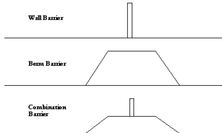
**Figure 16. Wall, berm and combination noise barriers**
