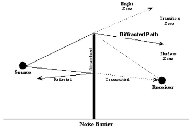
**Figure 8. Barrier absorption, transmission, reflection, and diffraction**
