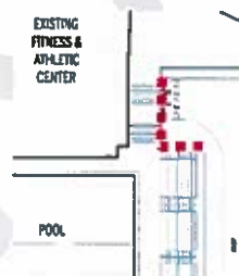
Figure A: Location where an increased barrier height may lower Main Circle event noise at Receiver C (Shown in Red)
