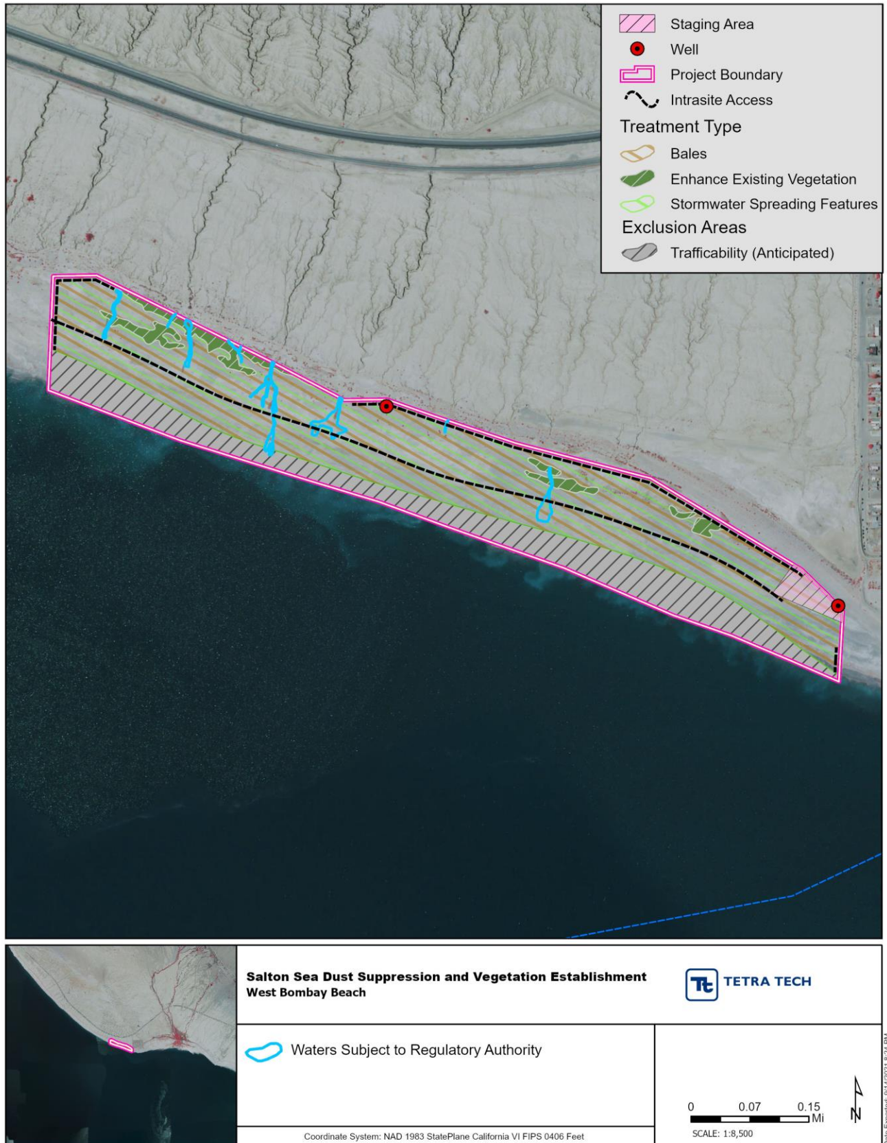
Figure 7. Bombay Beach West Site Project Implementation Plan
