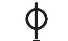
Common style appropriate for many uses; one point of ground contact. Compared to inverted-U racks, these are less prone to unintended perpendicular parking. Products exist for converting unused parking meter posts.
