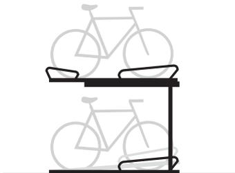
Typically used for high-density indoor parking. Performance varies widely. Models for public use include lift assist for upper-tier parking. Recommend testing before purchasing. Creates safety concerns not inherent to on-ground parking, and requires maintenance for moving parts.
