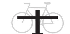
These racks are intended to capture a bike's frame and both wheels with a pivoting arm. In practice, they accommodate only limited bike types and have moving parts that create unneeded complications.
