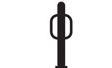
This style typically does not appropriately support a bike's frame at two separate locations.
