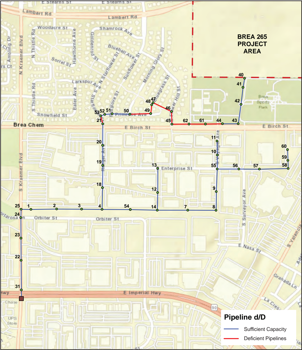
Figure 5.19-3 - Deficient Sewer Reaches with Project 5. Environmental Analysis
