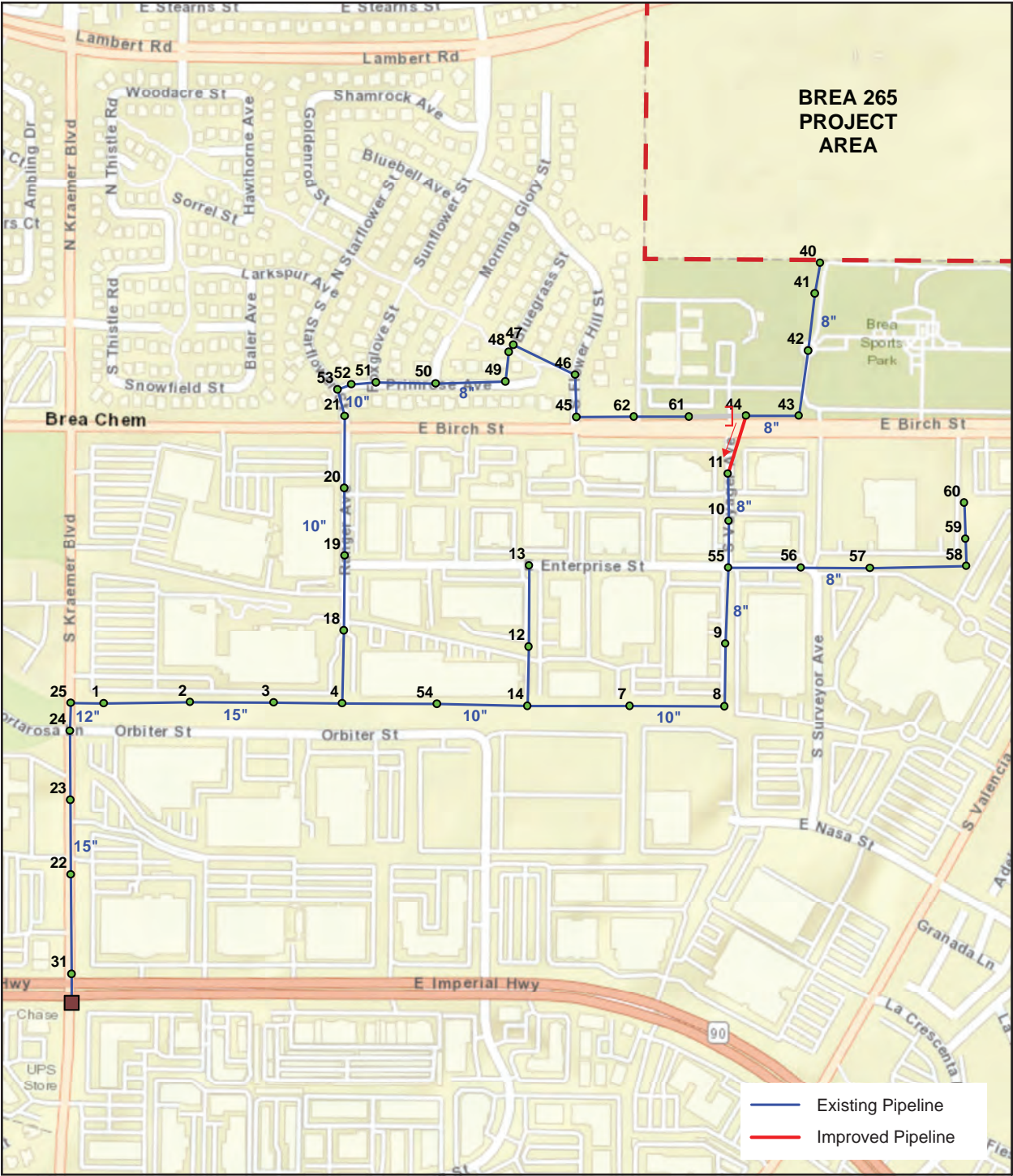
Figure 5.19-4 - Recommended Sewer Improvement Option 1 5. Environmental Analysis
