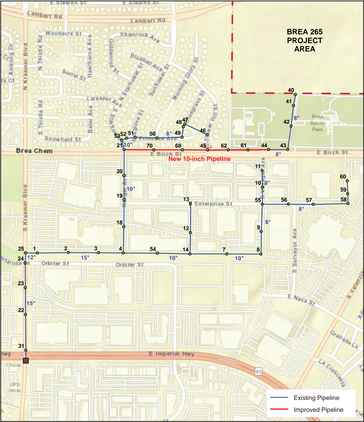
Figure 5.19-5 - Recommended Sewer Improvement Option 2 5. Environmental Analysis
