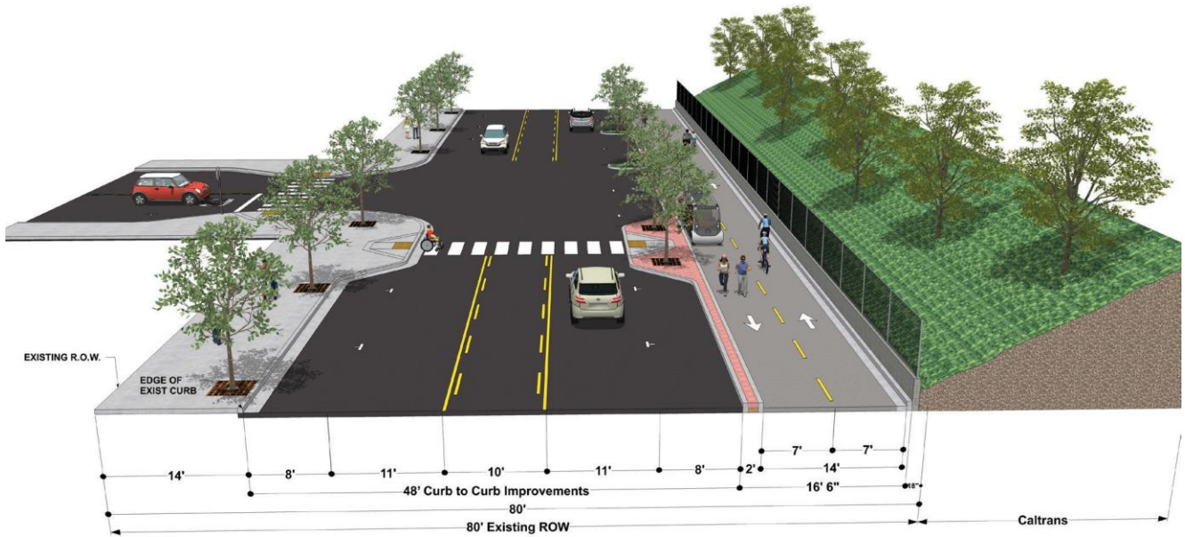
Figure 4-14: Option A - Parallel Parking and Multi-Use Path
