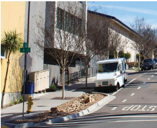
Existing parallel parking and curb extension
