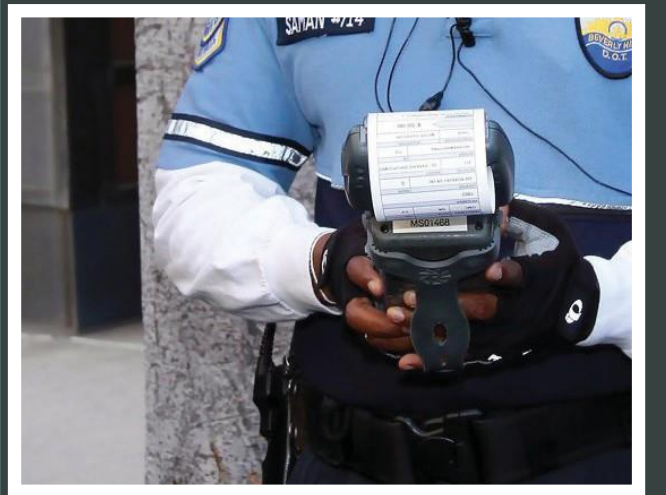
Parking Enforcement Handheld Device
