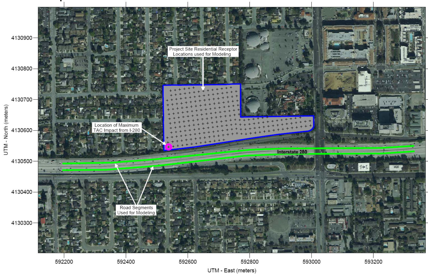
Figure 3. Project Site, On-Site Sensitive Receptors, Roadway Segments Modeled and Receptor with Maximum TAC Impacts
