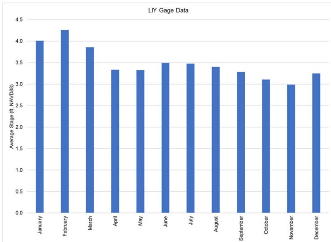
Based on the gage data presented above, BCI used an average WSE = 3.5 feet for EOC analysis. In addition, BCI evaluated one model for the EOC slope stability using the DWSE. The SAR panel suggested we also evaluate EOC at the DWSE because new regulations may include this requirement.
