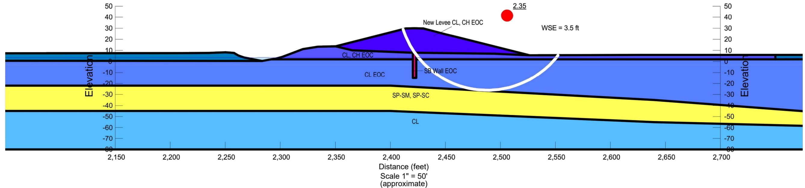
**Material ID and Type, Unit Weight, Undrained Shear Strength, Effective Cohesion, Effective Friction Angle**
