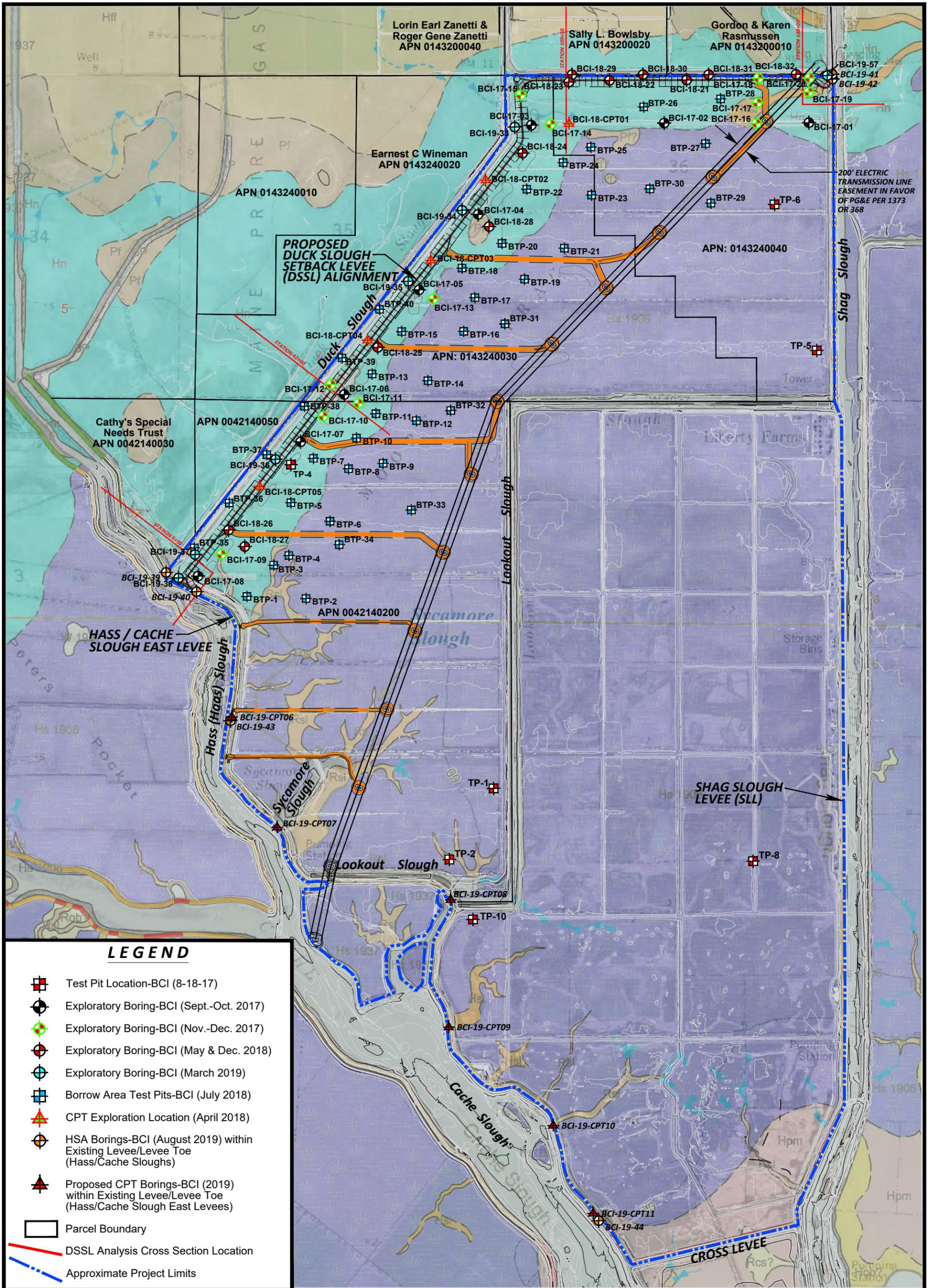
**FIGURE 3A, EXPLORATION SITE PLAN**
