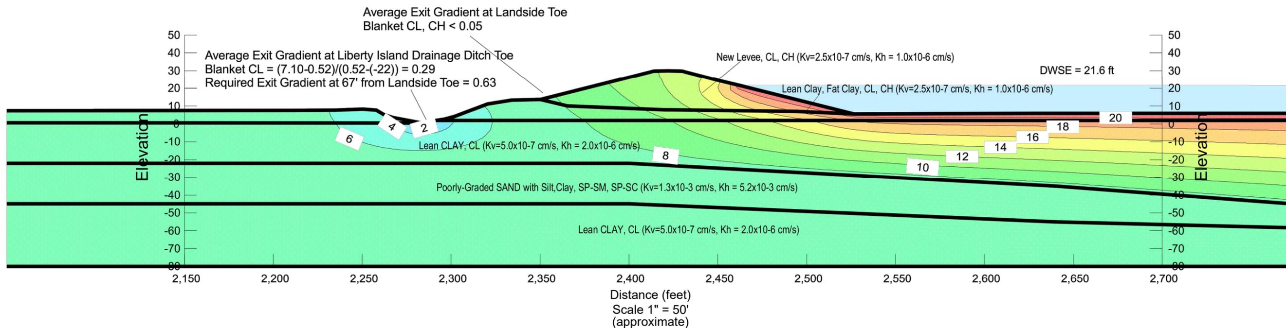
**Material ID and Type, Hydraulic Conductivity (Kh), Anisotropic Ratio (Kv/Kh)**
