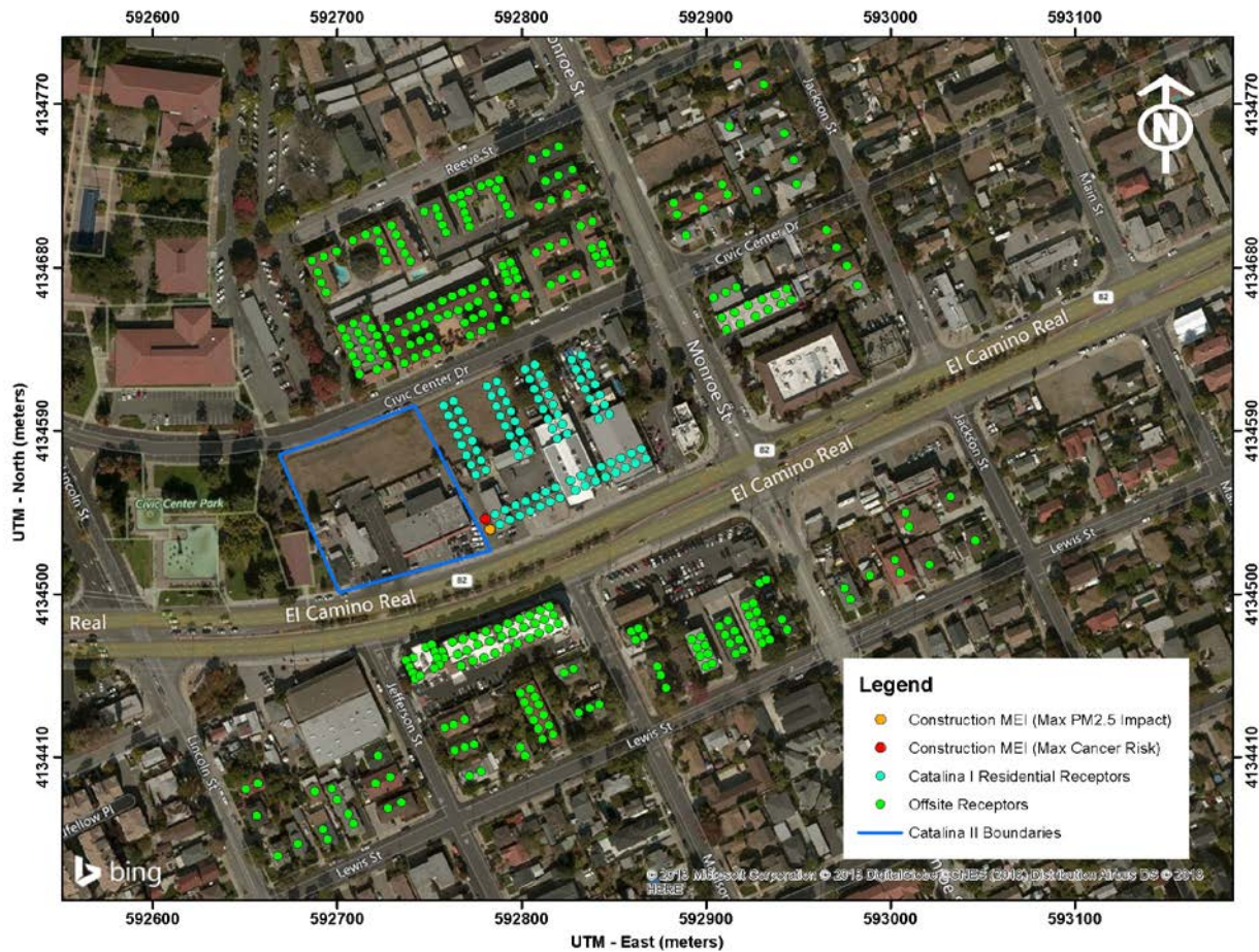
Figure 3. Project Construction Site and Locations of Off-Site Sensitive Receptors and Maximum TAC and PM 2.5 Impacts
