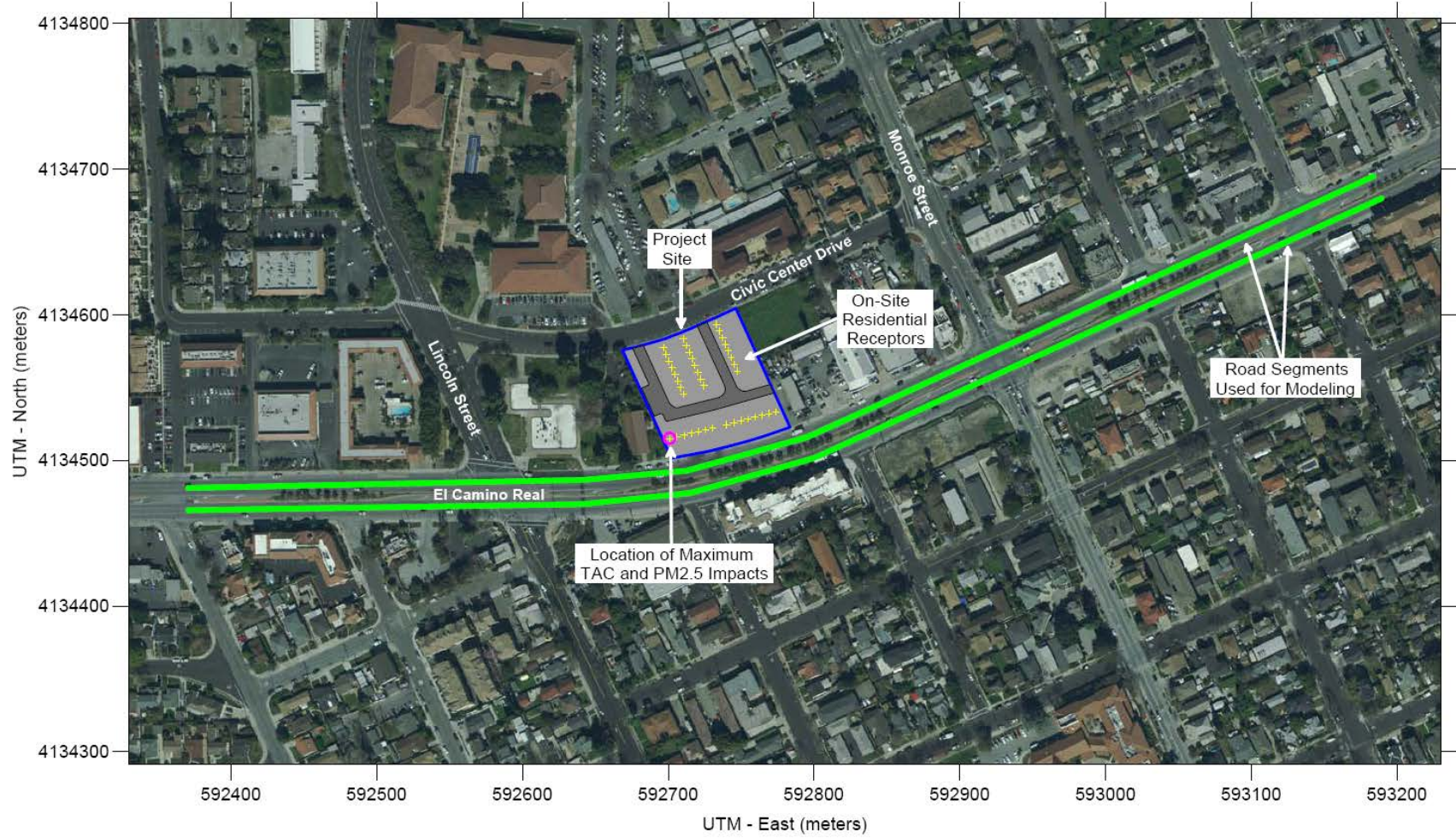
Figure 2. Project Site, On-Site Sensitive Receptors, Roadway Segments Modeled, and Receptor with Maximum Cancer Risk and Annual PM 2.5 Concentration
