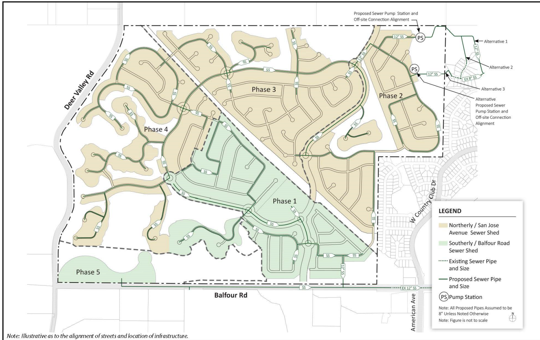
Figure 8 Existing and Proposed Sanitary Sewer
