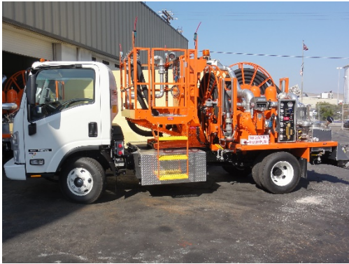
Typical LAWTFC Electric rechargeable hydrant fueling cart.
