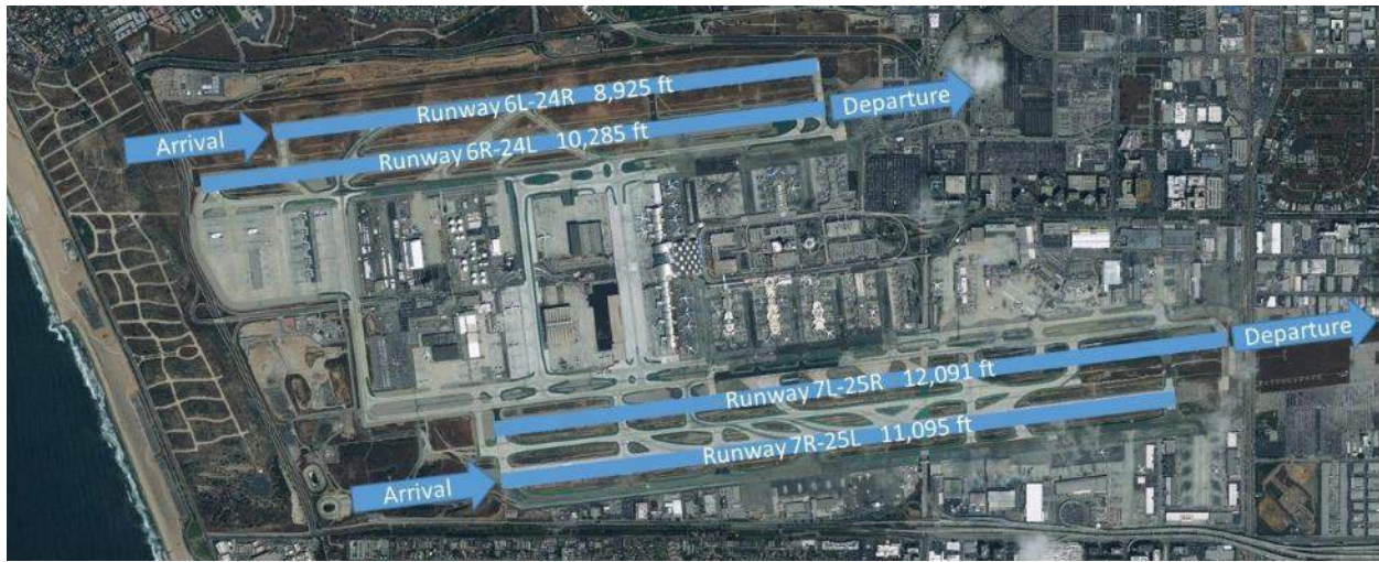
FIGURE 2-6: EAST FLOW OPERATIONS
