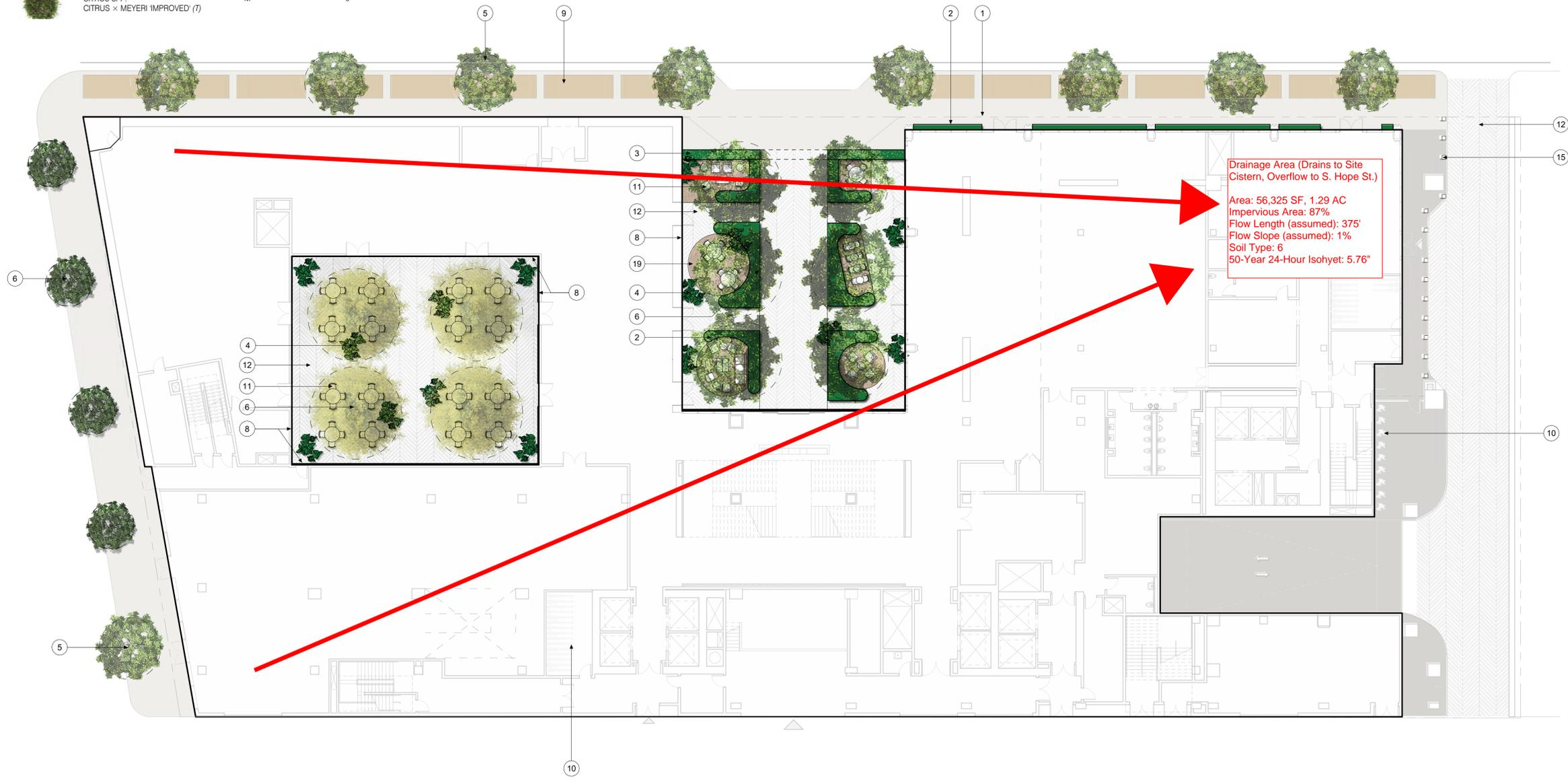
Drainage Area (Drains to Site Cistern, Overflow to S. Hope St.)
