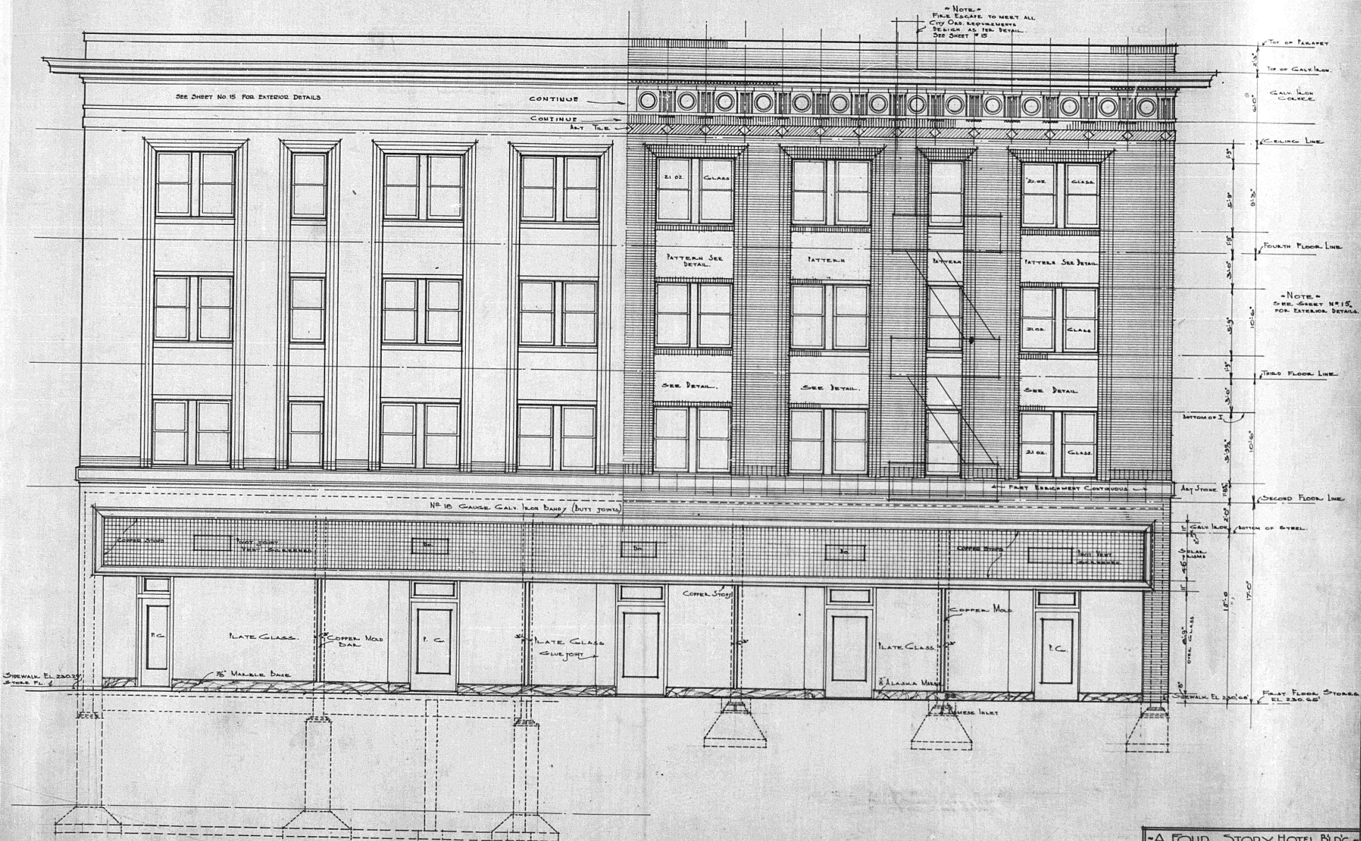
"PICO STREET ELEVATION" SCALE = 1/4" TO 1" NOTE - CONTRACTOR TO TAKE ALL EXTERIOR DETAIL FROM SHEET # 15
