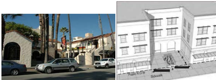
Forecourt Example - a brick wall and metal gate form the forecourt for this building, comprising 1/3 of the building's facade.
