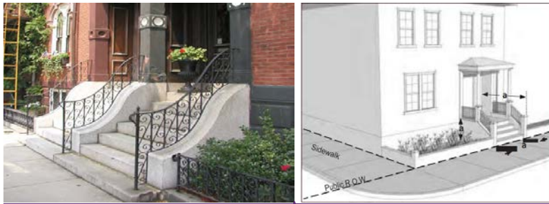
Stoop Example - stairs, landing, and landscape area of a typical stoop. Stoop diagram- elements and dimensions making up the Stoop frontage type.
