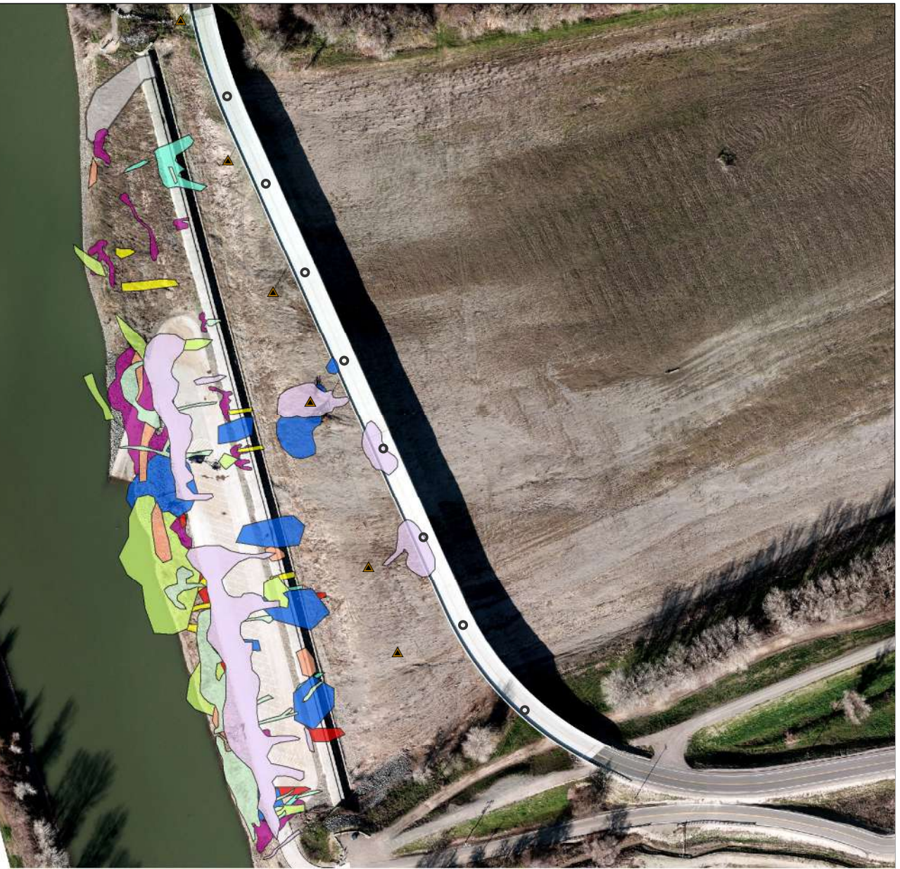
Figure 2 Large Wood Debris Locations During Spill Events
