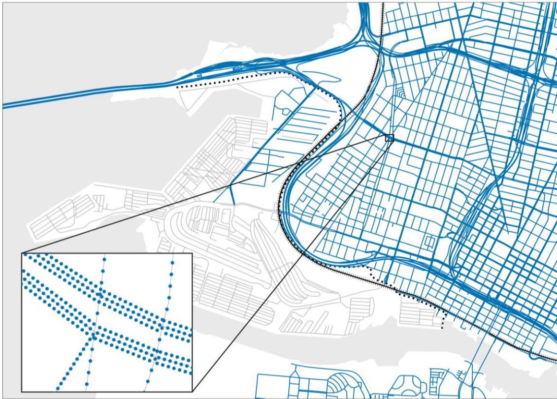
Figure 3-4. Locations of adjacent volume sources used to model emissions from on-road mobile sources. In the inset, the grey lines represent the location of roadways centerlines. The location of the marker represents the centroid of the volume source; the size of the marker does not reflect the dimensions of the volume source.
