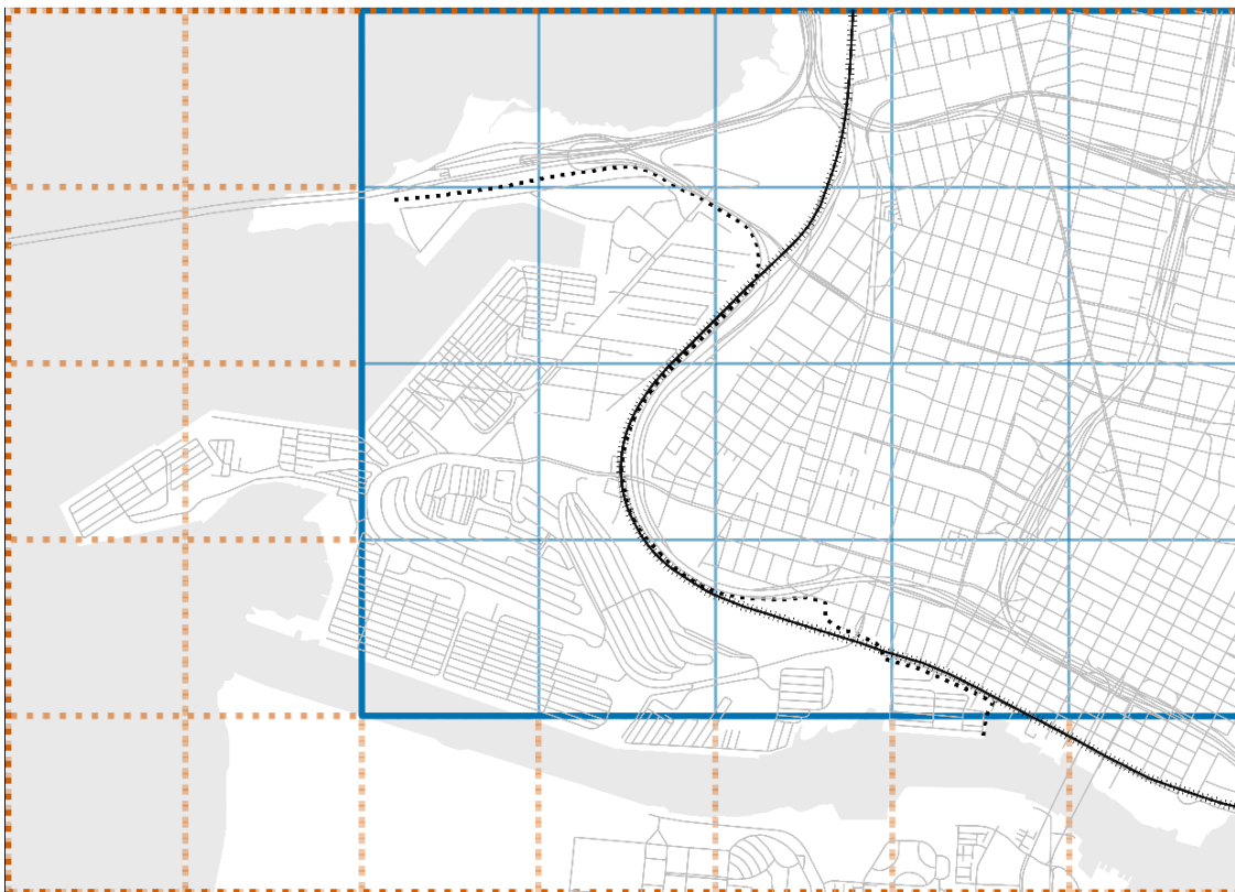
Figure 3-3. Extents of the Source Domain (red dotted lines) and Receptor Domain (blue solid lines) used in AERMOD modeling. The inner tiles represent the 1 km × 1 km grid cells of the regional modeling.
