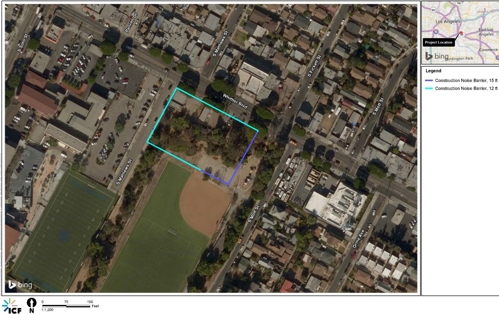
Figure 7. Location of Temporary Construction Noise Barriers
