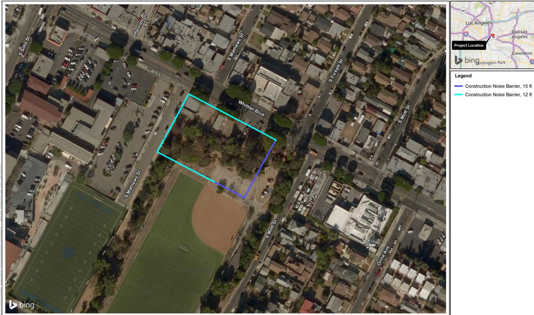
Figure 4-1. Location of Temporary Construction Noise Barriers
