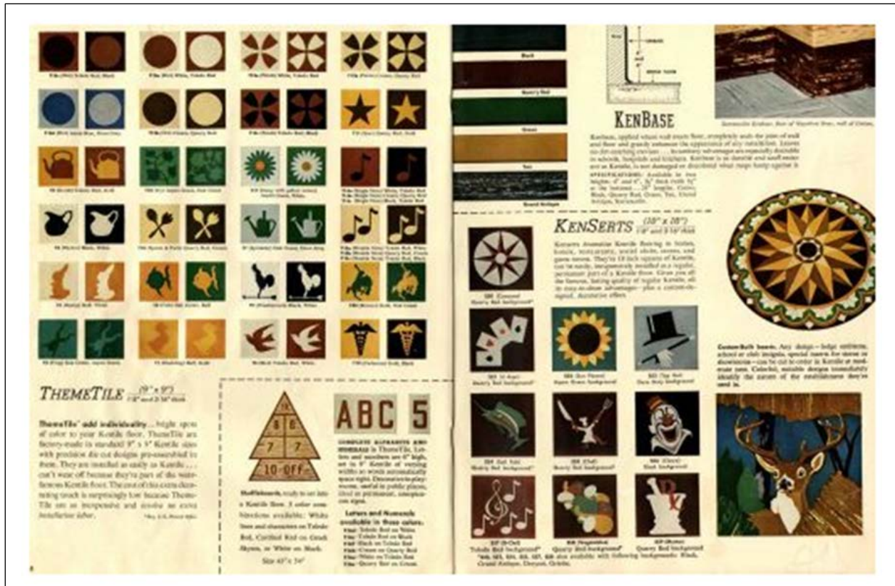
Figure 47. Kentile vinyl-asbestos flooring catalog, 1952, featuring tile patterns (e.g., pitcher, swallow, bunny, frogs, marlin, chef, clown) identical to those found in the Meridian School Kindergarten (Inspectapedia.com [n.d.]).
