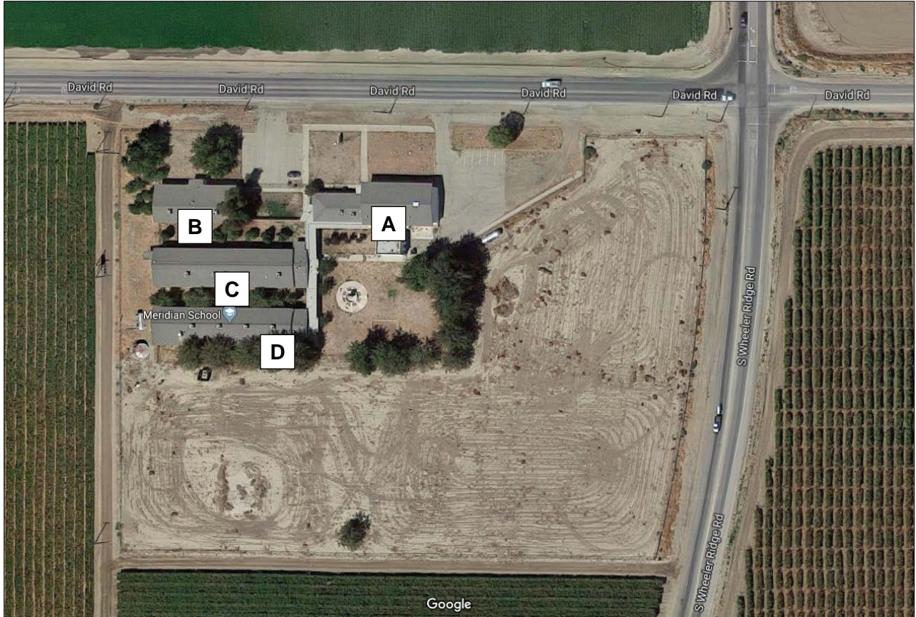
Figure 11. Google aerial view of former Meridian School campus, showing “finger-plan” layout of campus buildings.
