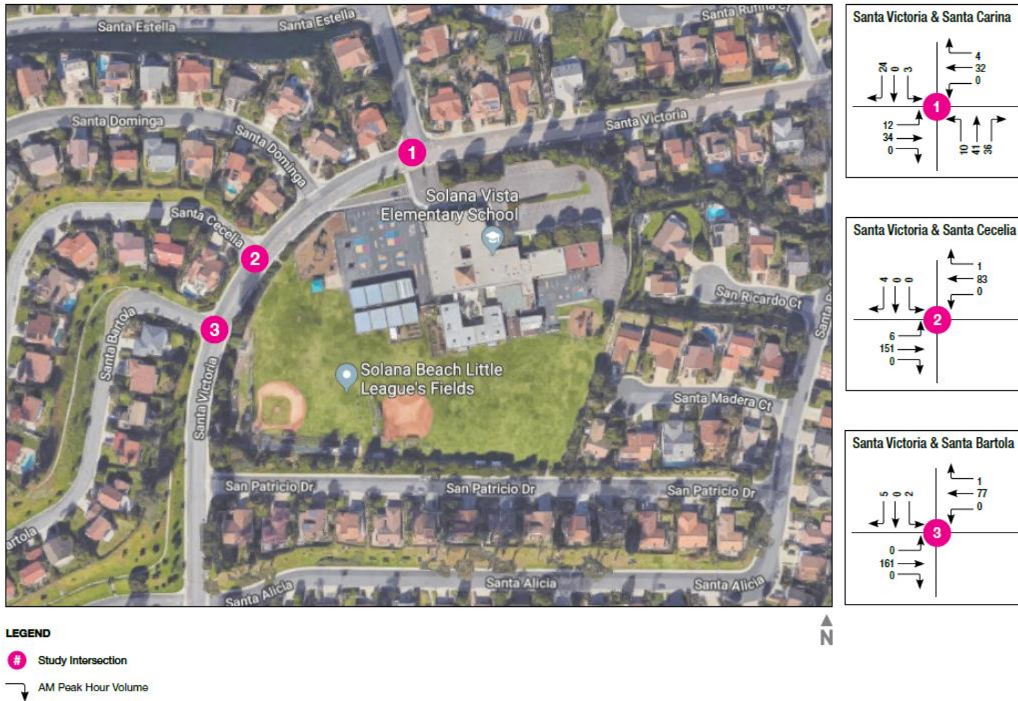
FIGURE 8: EXISTING YEAR (2018-19) WITH PROJECT VOLUMES – AM PEAK HOUR
